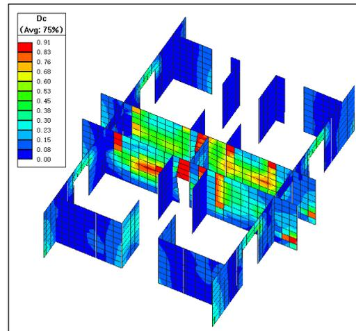
(a) Damage distribution on the first-floor shearing wall
