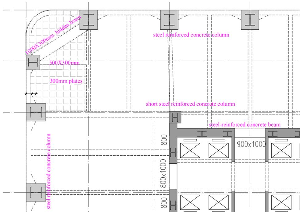
Fig. 4 Schematic diagram of structural characteristics
