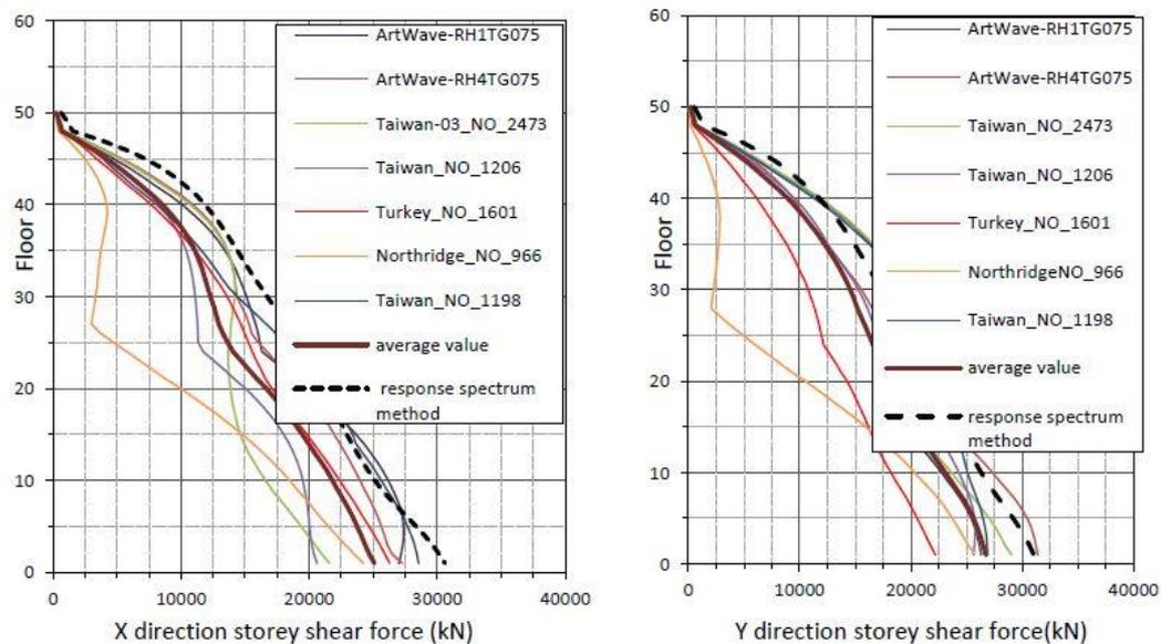
Fig. 5 Storey shear forces
