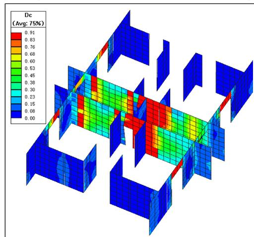
(b) Damage distribution on the third-floor shearing wall
