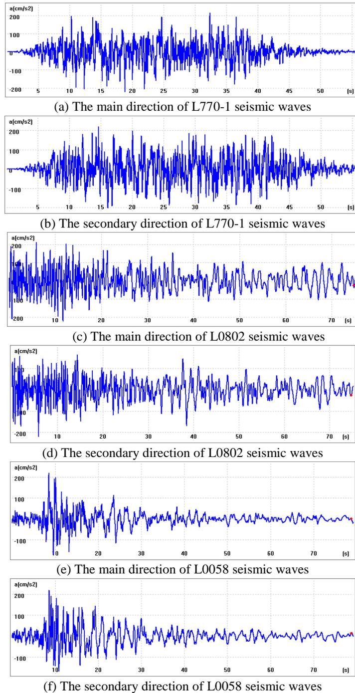
Fig. 11 Time history curve of seismic waves
