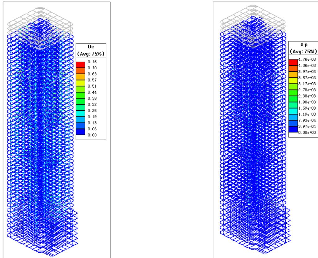
Fig. 16 Compressive damage to concrete beams and plastic strain distribution of rebar
