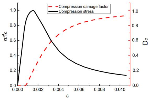
Fig. 12 The relation diagram between damage factor and stress-strain curve of concrete
