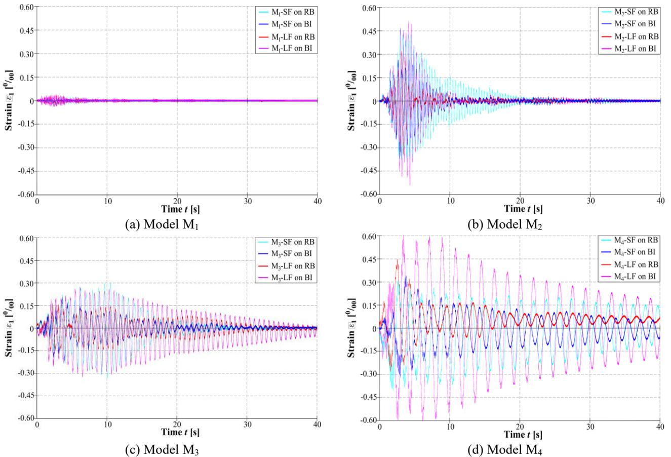
Fig. 14 Vertical strain on the right bottom side of the steel column  $\epsilon_1$  for accelerogram ABL
