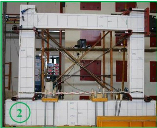
(a) End of loading step 2: Slight hairline flexural cracks in beam
