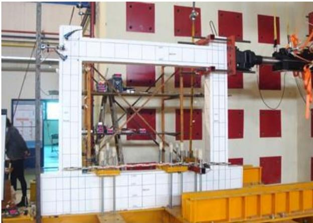
(b) Test rig and instrumentation of the cyclic test
