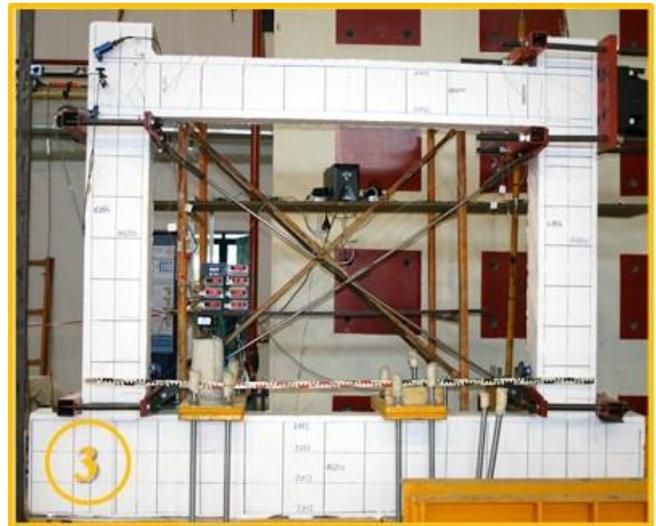
(b) End of loading step 3: Flexural cracks in beam and columns and hairline diagonal cracks in joints
