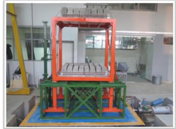
(b) photo of the test steel frame on shaking table
