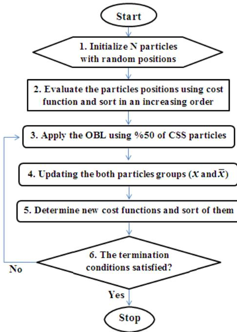
Fig. 1 The flowchart of OBLCSS algorithm
