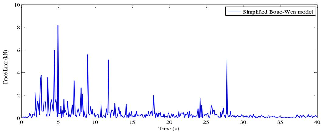
Fig.10 Time history of damper force error for proposed simplified model
