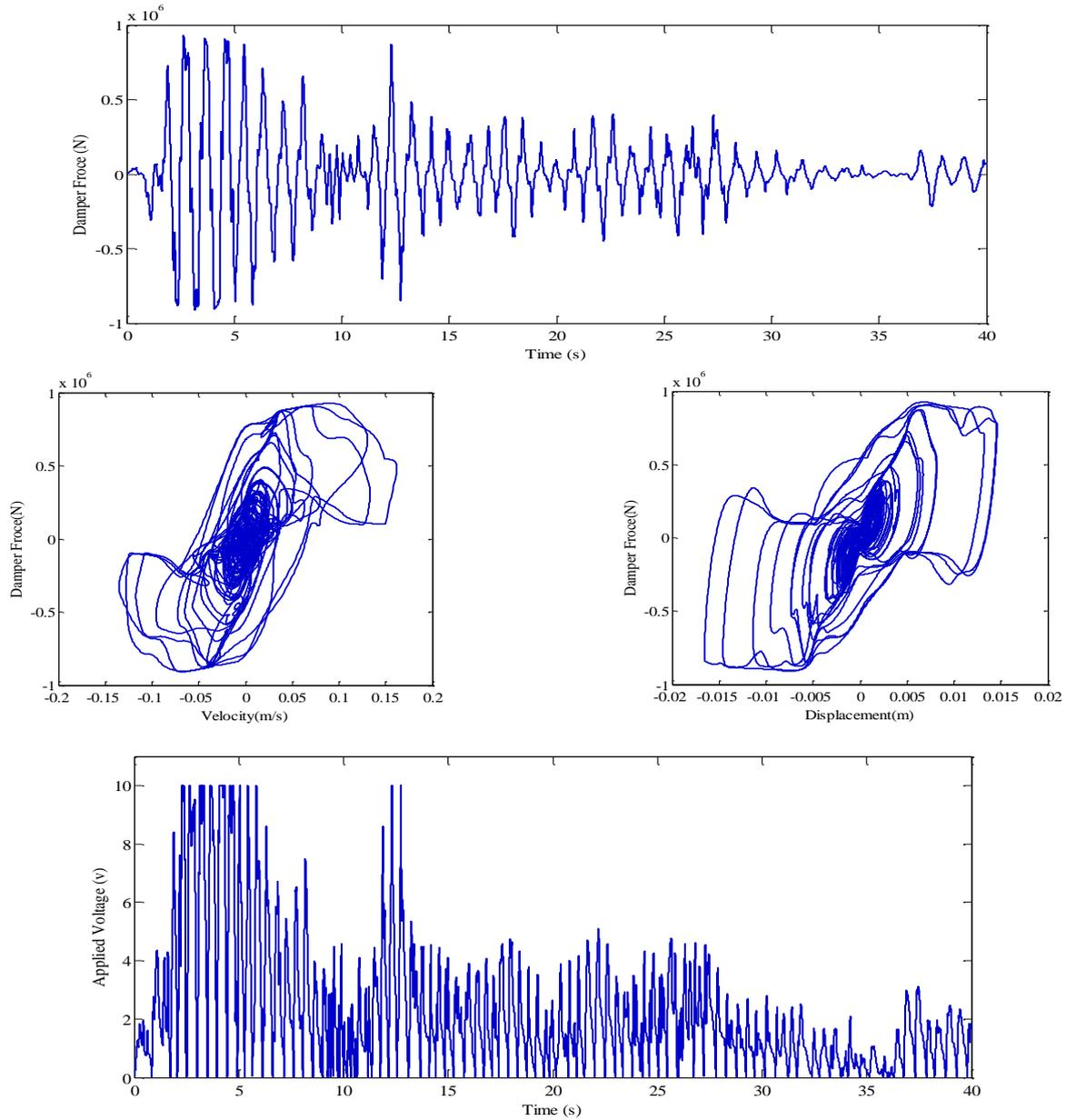
Fig. 3 Numerically generated experimental data for the modified Bouc-Wen model of 1000 kN MR damper under the fuzzy logic controller simulation
