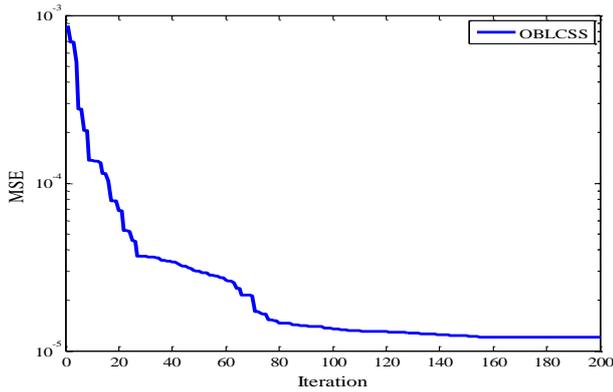
Fig. 8 Convergence history of MSE for proposed simplified Bouc-Wen using OBLCSS
