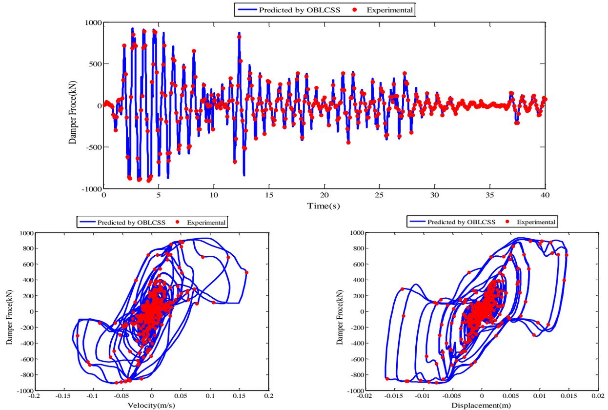
Fig. 5 Comparison of experimental and predicted damper responses with modified Bouc–Wen model with FLC signal
