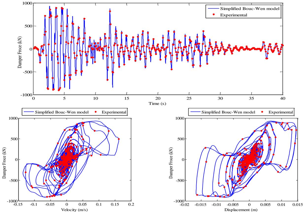
Fig. 9 Comparison between experimental and predicted damper responses with propose simplified Bouc-Wen model with FLC signal
