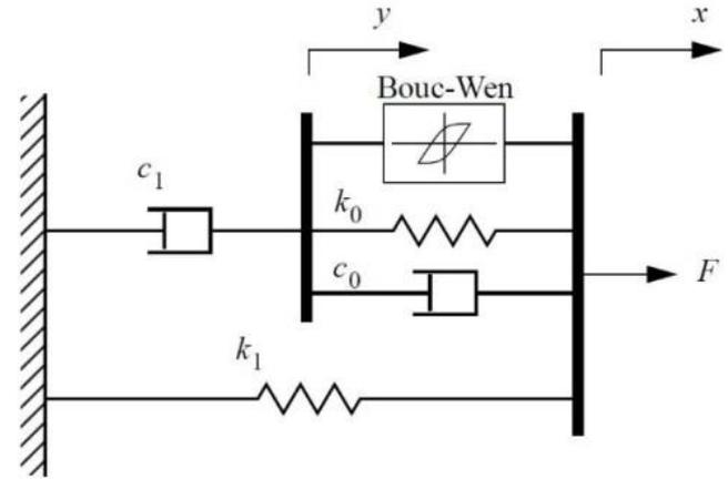
Fig. 2 Modified Bouc-Wen model of MR damper
