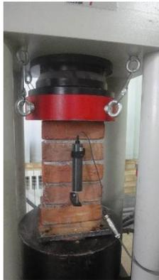
(c) Test setup of prism masonry
