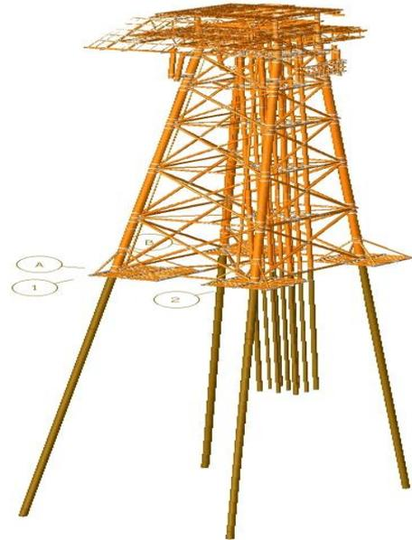
Fig. 5 Piles are enclosed inside the jacket leg
