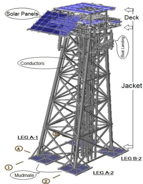
Fig. 4 3D finite element model of substructure and topside
