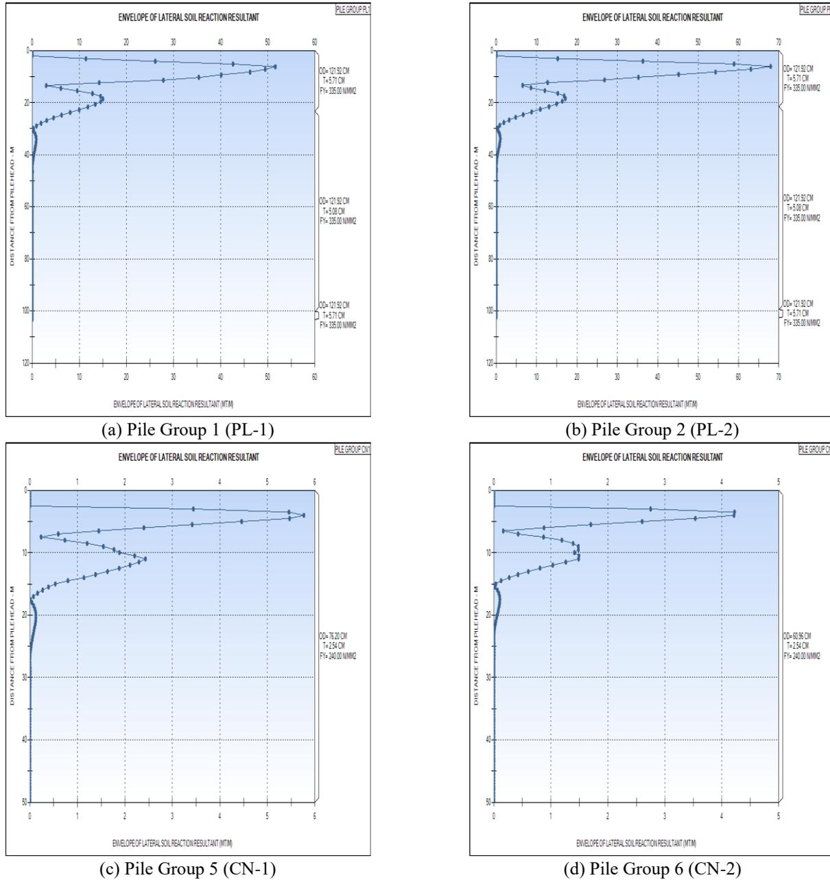
Fig. 13 Envelope of lateral soil reaction resultant for piles groups vs depth from PILEHEAD level
