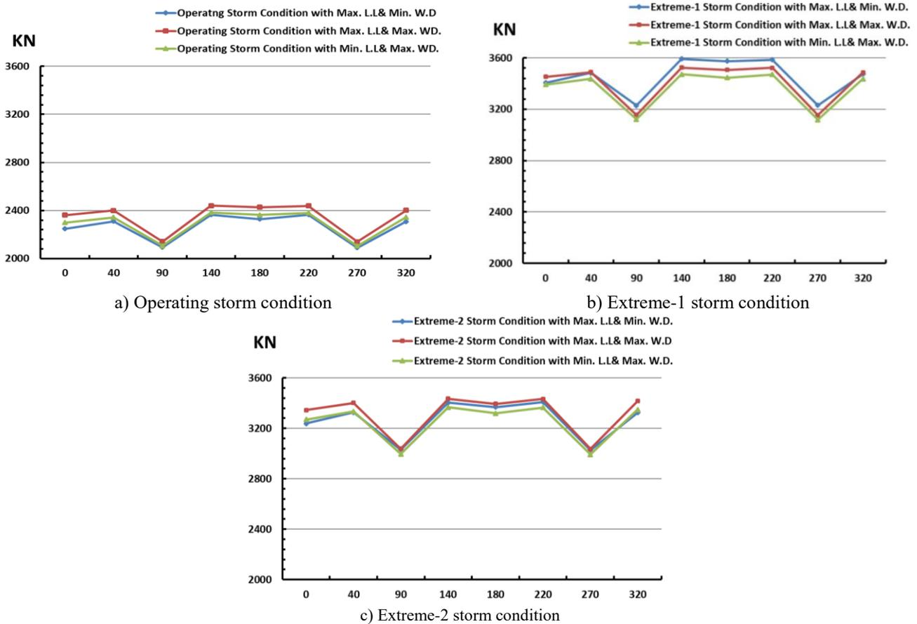
Fig. 7 Total applied horizontal loads for different incidence angles of the environmental loads' direction
