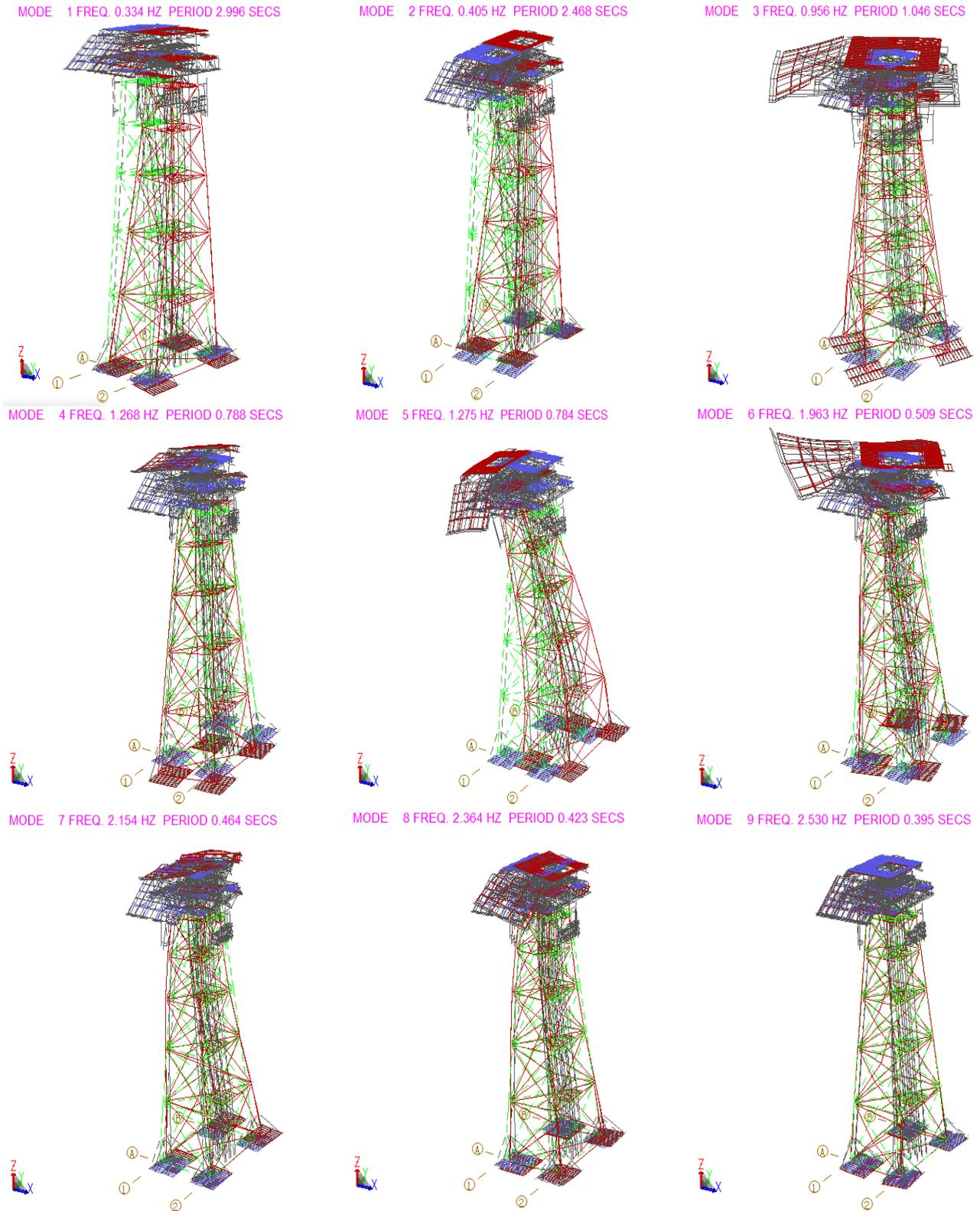
Fig. 6 First nine mode shapes and natural frequencies of the platform at site
