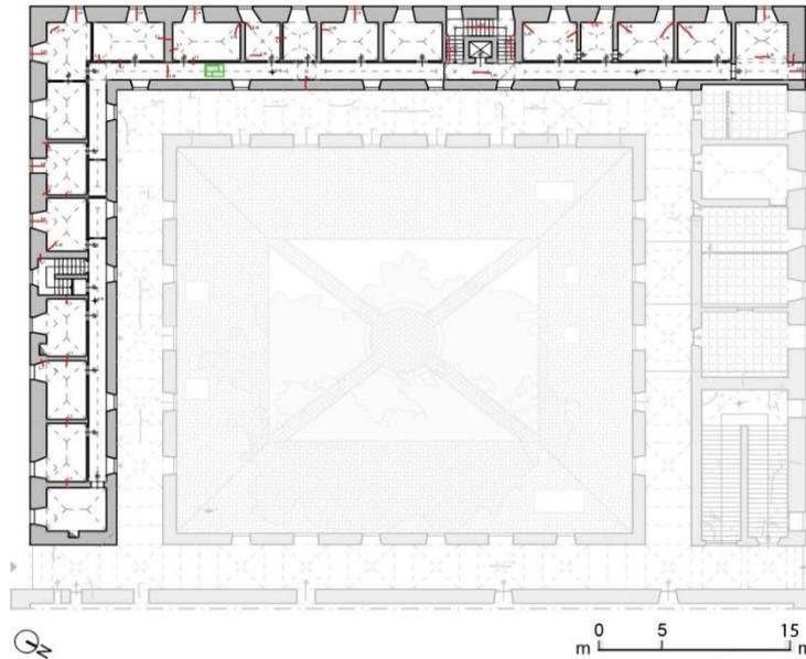
(a) Plan of the mezzanine floor; in red is characterized the cracking pattern and in green is reported the location of the visual investigation on a wall declaring the presence of masonry in solid bricks and lime mortar
