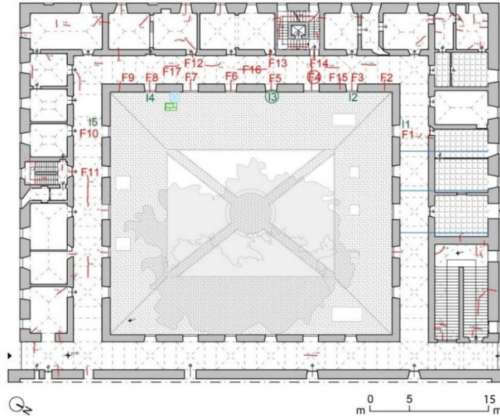
(a) Plan with the cracking pattern (red lines) and location of the monitoring instruments: F1-F17 crackmeters, I1-I5 inclinometers; in pale blue and green the inspections on mortar and masonry respectively; in blue lines the tie rods installed after 1997 earthquake
