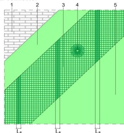
(b) Sequence of the different work phases in elevation;  $L_s$  is the length of overlap for the net bands
