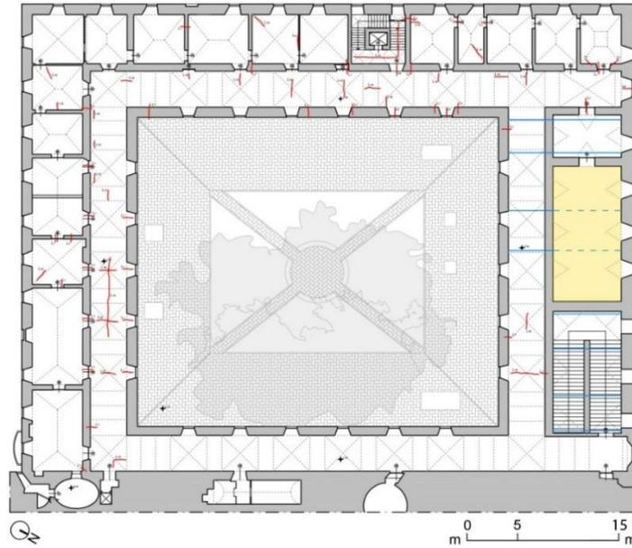
(a) Plan of the first floor; in red is characterized the cracking pattern, in blue lines the tie rods installed after 1997 earthquake; the region in yellow highlights the “PhD’Room”
