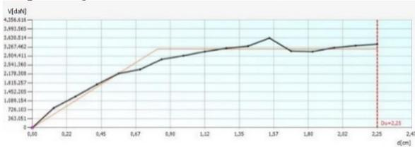
(b) Pushover analysis conducted in direction -Y for static forces seismic load distribution (black lines) and the corresponding bi-linear curve (red lines)
