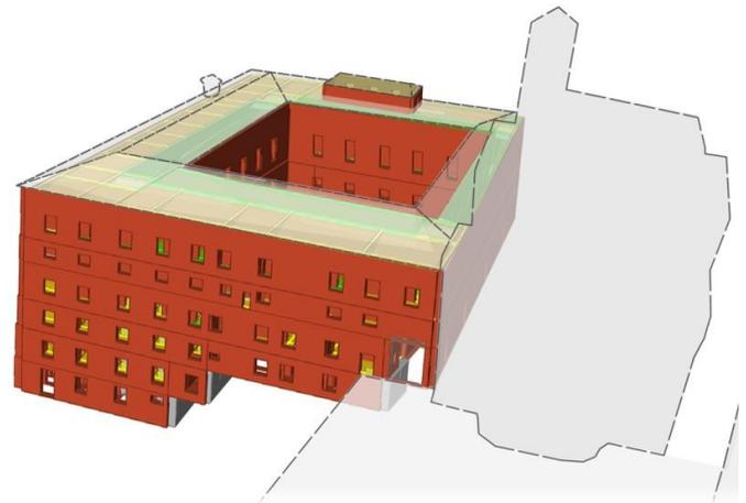
(a) Plan of the numerical model, the interior walls relative to different floors are overlapping, n.7 is the “reference node” of the roof-floor used in the pushover analysis
