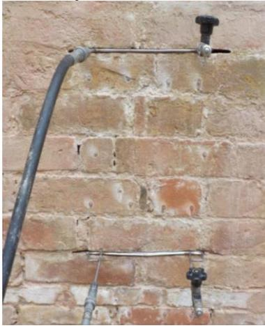
(b) Execution of the MP 2 compression test with flat jacks in order to establish the maximum compression strength ( $f_m$ ) and the Young's module ( $E$ ) of the brick wall
