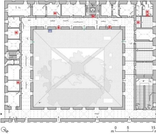
(a) Position of the experimental tests conducted on the ground floor: in red the video endoscopy from intrados, in green the performed drills, in blue the location of the performed double flat jack test
