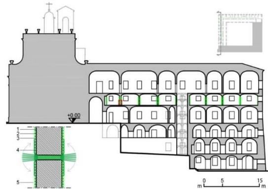
a) Cross-section: in green are characterized the F.R.C.M. applied at the mezzanine floor; on the left side there is a technical detail of the reinforced plaster with fiber transversal connector
