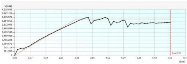
(a) Pushover analysis conducted in direction -X for uniform seismic load distribution (black lines) and the corresponding bi-linear curve (red lines)
