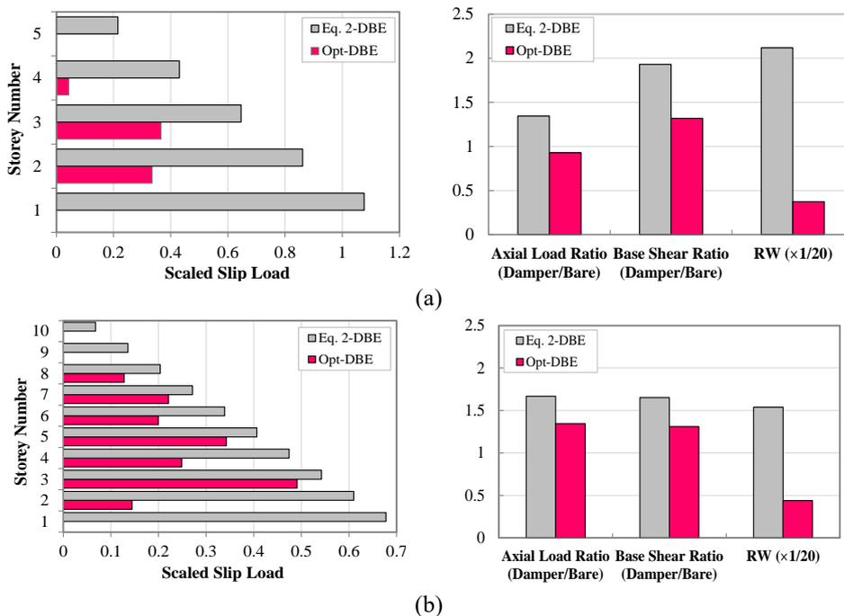
Fig. 5 Slip load, column axial load and base shear ratios for (a) 5-storey and (b) 10-storey frames with optimised friction walls and those designed based on Eq. (2), DBE event
