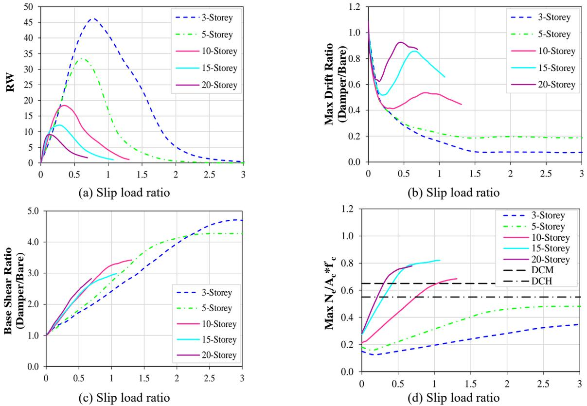
Fig. 3 Variations of (a)  $R_w$ , (b) maximum drift ratio, (c) base shear ratio, and (d) maximum  $N_e/A_c f_c$  for the 3, 5, 10, 15 and 20-storey frames as a function of slip load ratio, average of selected natural earthquakes
