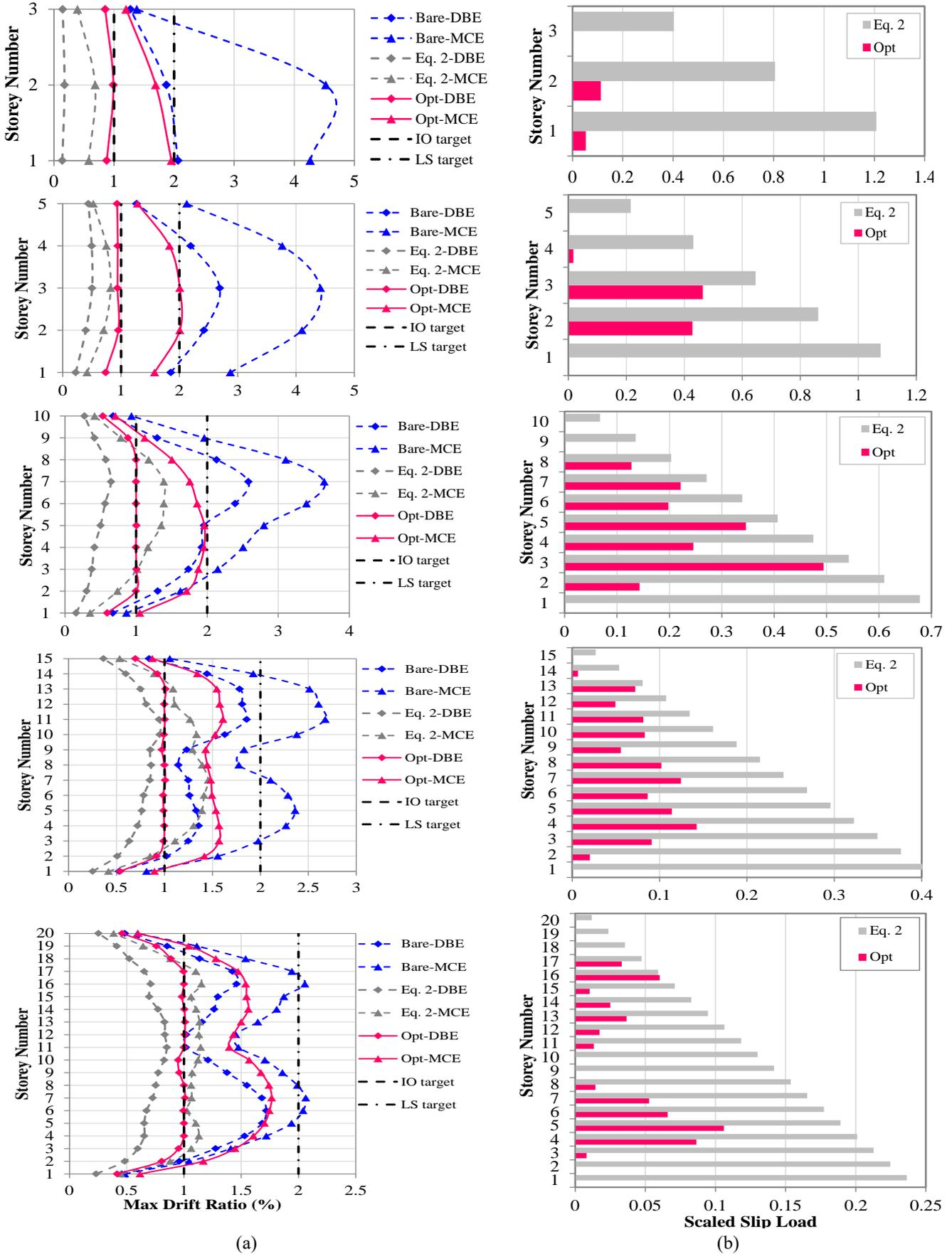
Fig. 7(a) Maximum drift ratios and (b) Slip load ratios for 3, 5, 10, 15 and 20-storey frames without wall and with optimised friction walls and those designed based on Eq. (2), DBE and MCE events
