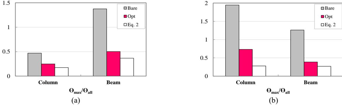
Fig. 6 Plastic rotation ratio (maximum to allowable plastic rotation) of the beam and column elements for (a) 5-storey and (b) 10-storey frames without friction wall, with optimised friction walls and those designed based on Eq. (2), DBE event
