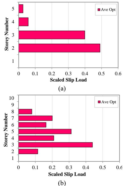
Fig. 10 Average optimum slip load values for (a) 5-storey and (b) 10-storey frames, Average of six synthetic DBE and MCE events
