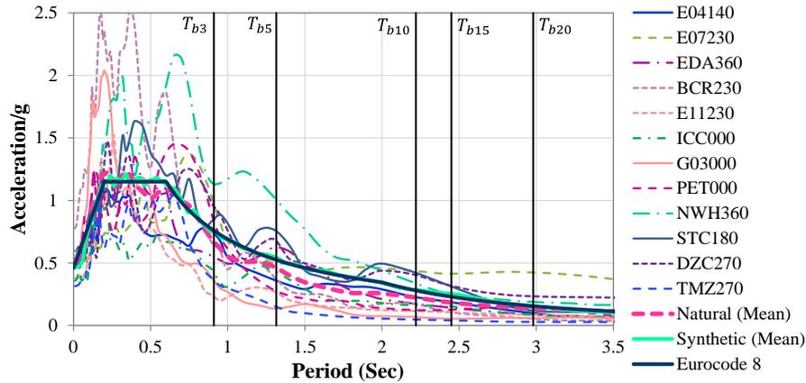
Fig. 2 Comparison between the elastic acceleration response spectra of the selected natural and synthetic earthquake records and the EC8 design spectrum, 5% damping ratio
