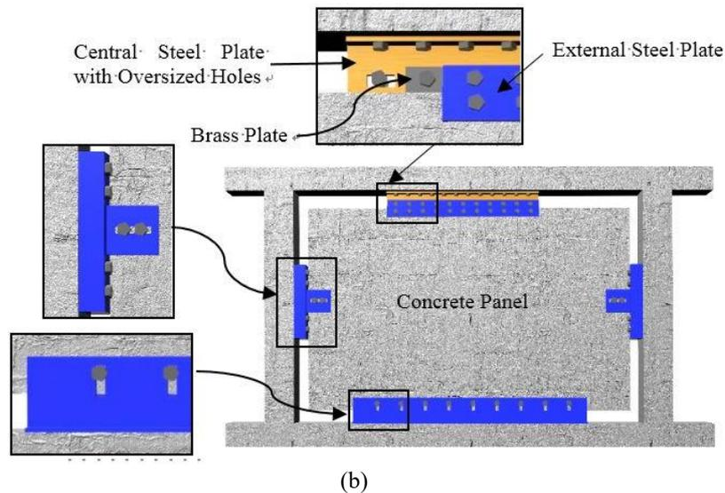
Fig. 1(a) Geometry of the reference RC frames equipped with friction wall dampers, (b) schematic view of the friction wall damper (adopted from Nabid *et al.* (2017))
