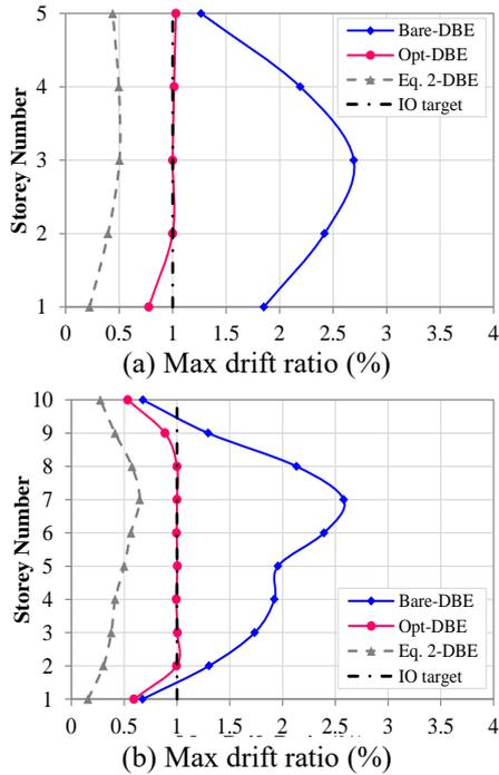
Fig. 4 Maximum drift ratios for (a) 5-storey and (b) 10-storey frames without friction walls (bare frame), with optimised friction walls and those designed based on Eq. (2), DBE event
