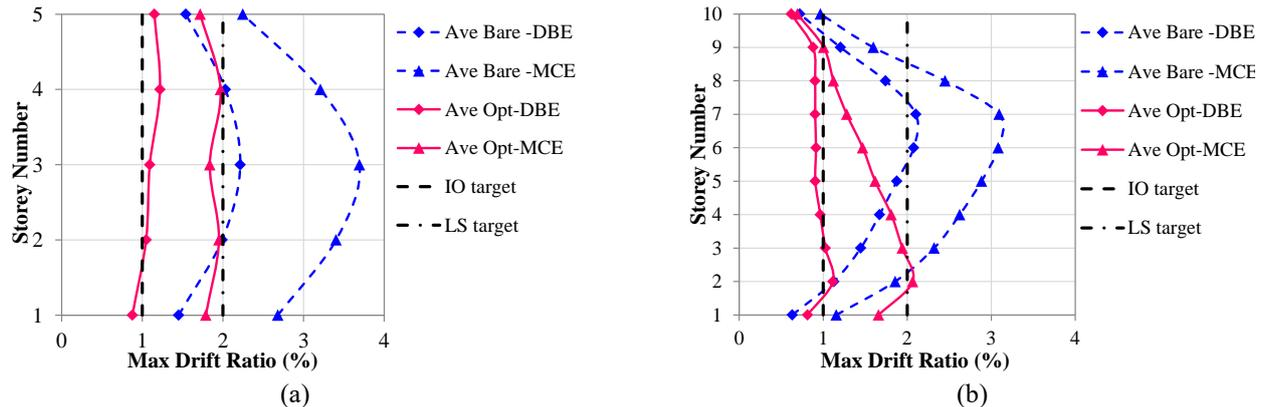
Fig. 11 Maximum drift ratios of (a) 5-storey and (b) 10-storey frames with optimised friction walls obtained for six synthetic DBE and MCE events, Average of twelve natural DBE and MCE events
