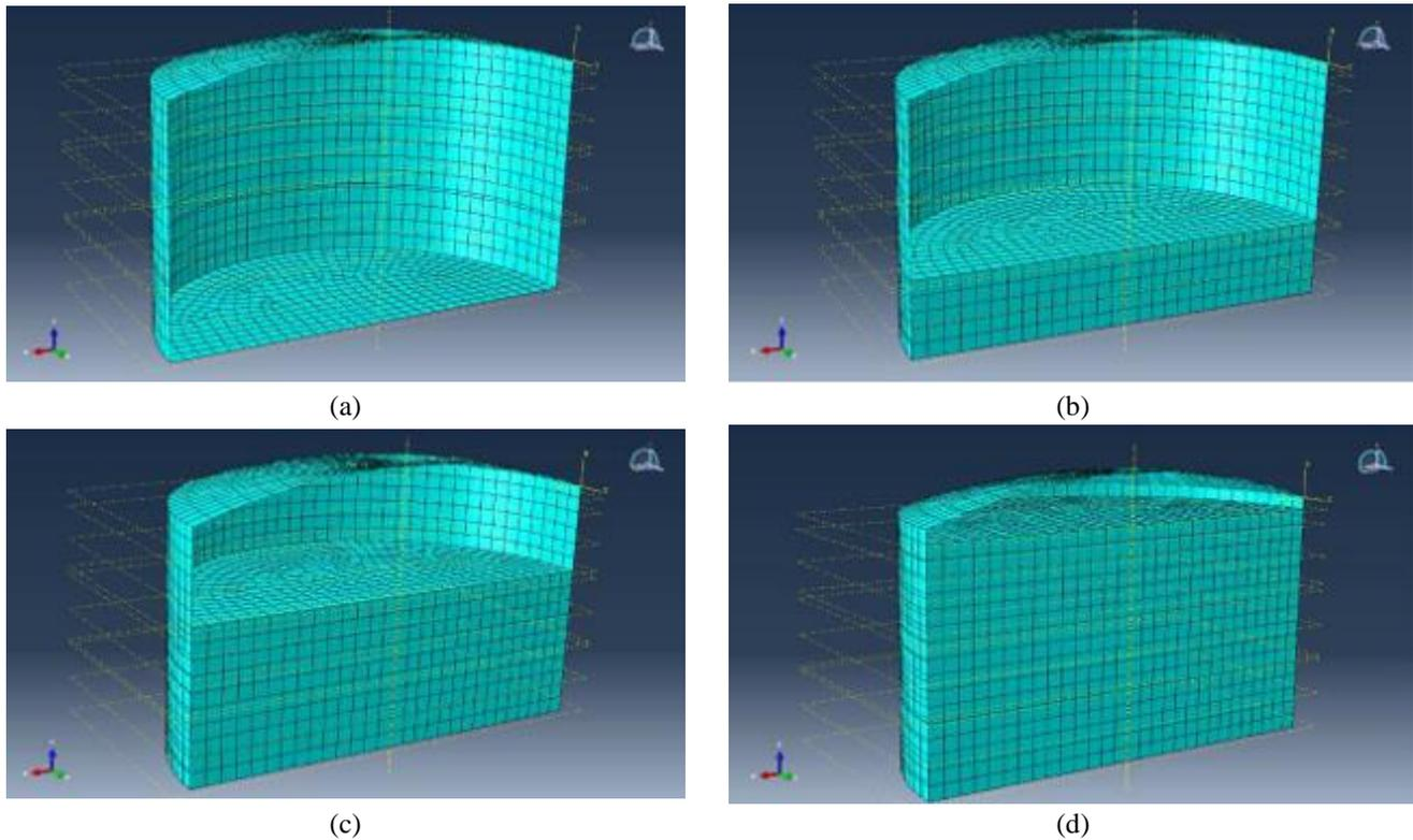
Fig. 3 Variants of liquid filling for tank with  $V=10,000 \text{ m}^3$
