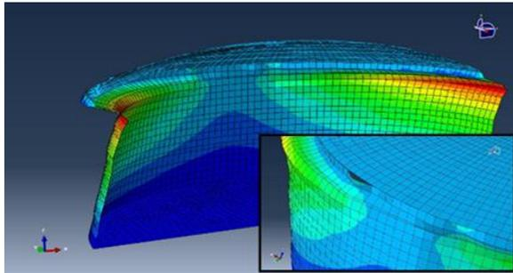
(c) Tank with circumferential cut of weld between shell and roof –  $f=0.556$  Hz
