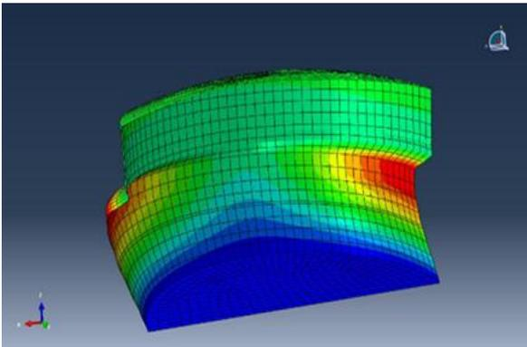
(c) Tank filled to 2/3 of allowable limit –  $f = 0.903$  Hz
