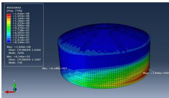
(c) Tank filled to 2/3 of allowable limit –  $t = 2.16$  s (max value: 184.60 MPa)
