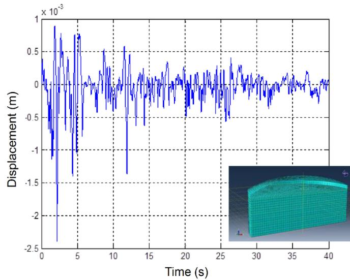
Fig. 15 Displacement UX time history for tank with  $V=32,000 \text{ m}^3$  filled to allowable limit under the non-uniform El Centro earthquake – reference node  $X_g$  (peak value:  $2.40 \cdot 10^{-3} \text{ m}$ )
