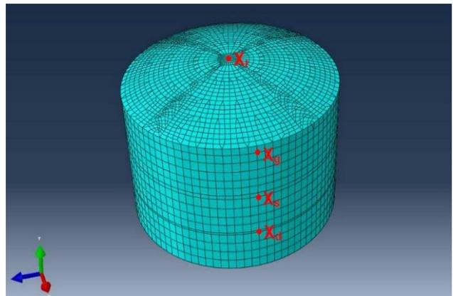
Fig. 2 FE model of steel tank with  $V=32,000 \text{ m}^3$
