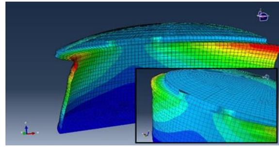
(d) Tank with circumferential cut of weld between shell and roof and with radial cut of weld in roof –  $f=0.556$  Hz
