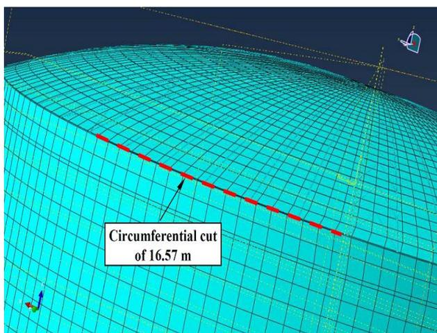
(a) Cut of weld between shell and roof
