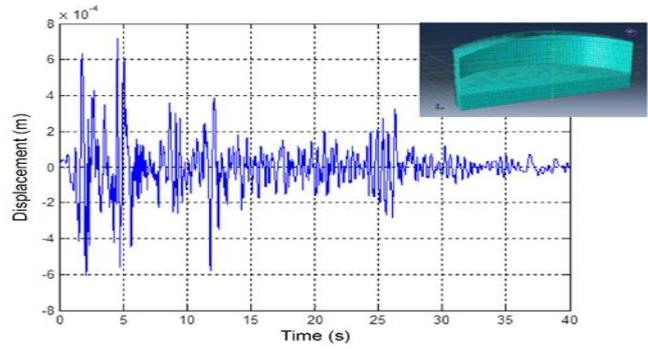
(b) Tank filled to 1/3 of allowable limit (peak value:  $7.20 \cdot 10^{-4}$  m)
