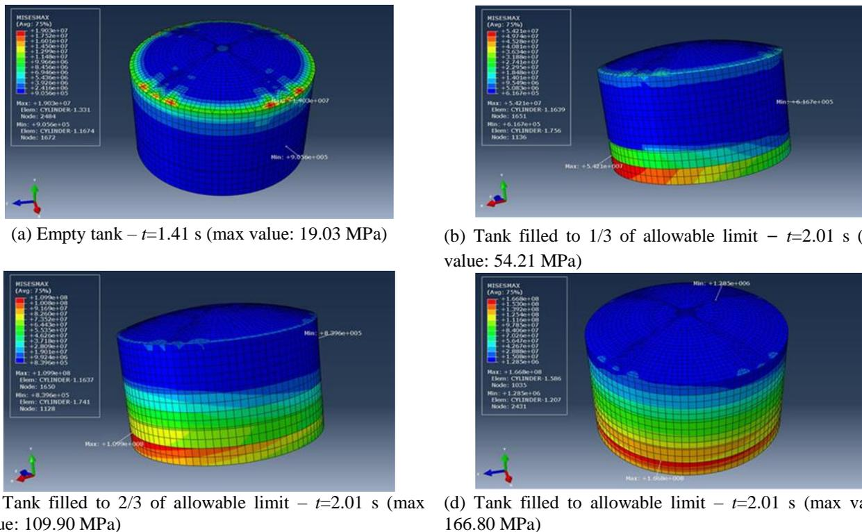
Fig. 11 Extreme distributions of von Mises stresses for tank with  $V = 10,000 \text{ m}^3$  under the uniform Polkowice 2002 mining tremor
