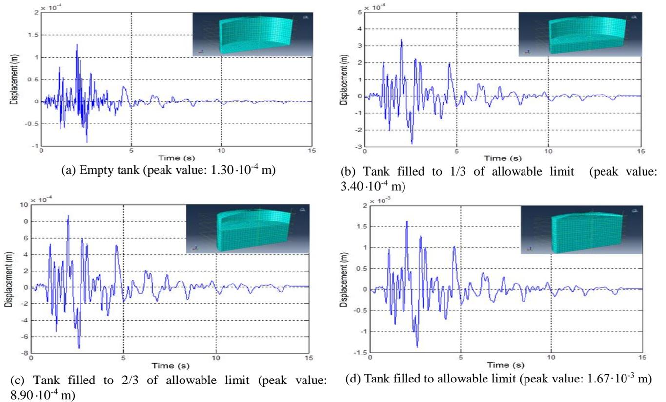
Fig. 10 Displacement UX time histories for tank with  $V=10,000 \text{ m}^3$  under the uniform Polkowice 2002 mining tremor – reference node  $X_i$
