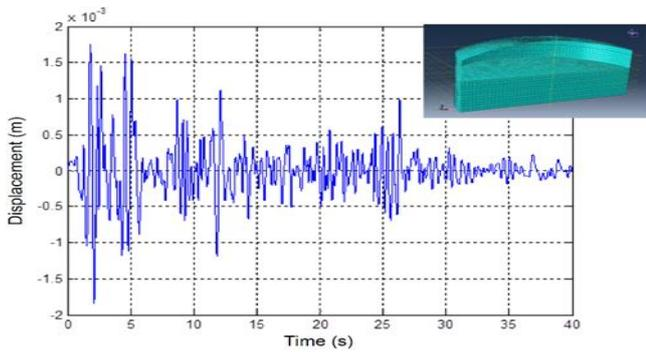
(c) Tank filled to 2/3 of allowable limit (peak value:  $1.80 \cdot 10^{-3}$  m)
