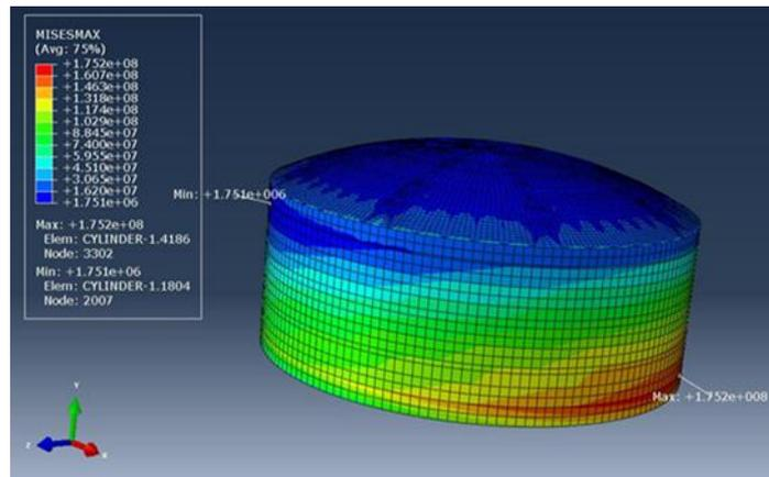
Fig. 16 Extreme distribution of von Mises stress for tank with  $V=32,000 \text{ m}^3$  filled to allowable limit under the non-uniform El Centro earthquake –  $t=2.19 \text{ s}$  (max value: 175.20 MPa)
