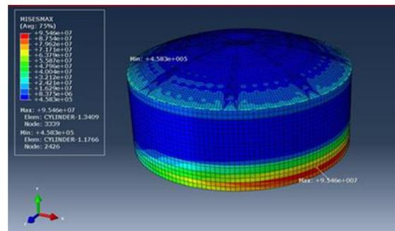
(b) Tank filled to 1/3 of allowable limit –  $t = 1.80$  s (max value: 95.46 MPa)
