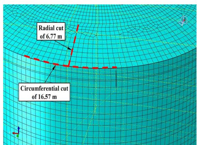
(b) Cut of weld between shell and roof and radial cut of weld in the roof
