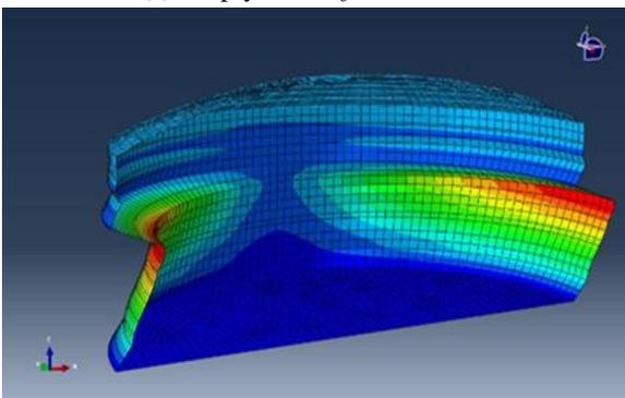
(c) Tank filled to 2/3 of allowable limit –  $f = 0.702$  Hz
