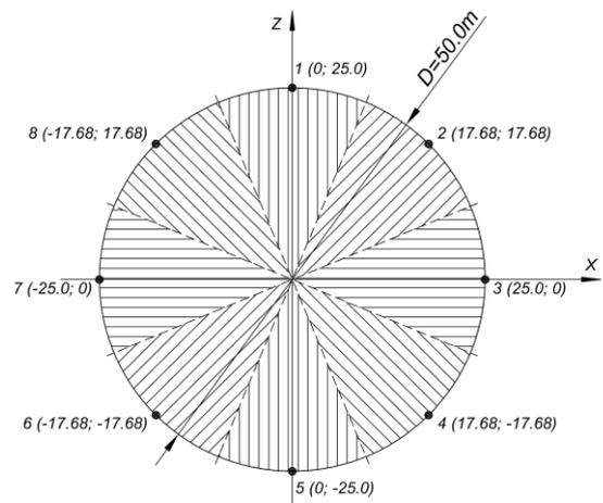
Fig. 14 Division of base plate of tank with  $V=32,000 \text{ m}^3$  for the purposes of generation of non-uniform excitation
