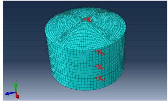
Fig. 1 FE model of steel tank with  $V=10,000 \text{ m}^3$
