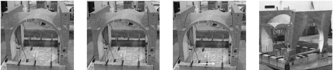
Fig. 16 Collapse mechanism of the vault NT for the seismic input of PTA=0.398 g, with the overturning of the side A and the development of a four-hinge mechanism on the vault
