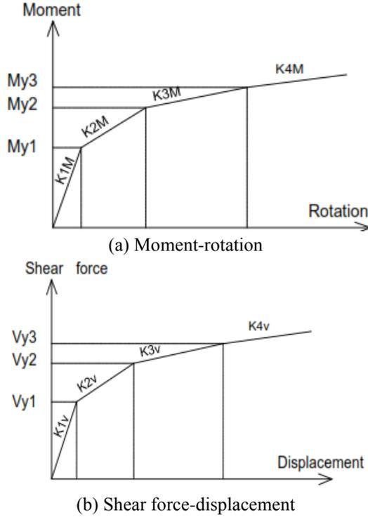
Fig. 3 Spring relationships used in steel connection
