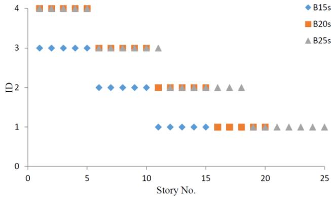
Fig. 1 Dimension ID of beams for different frames and stories
