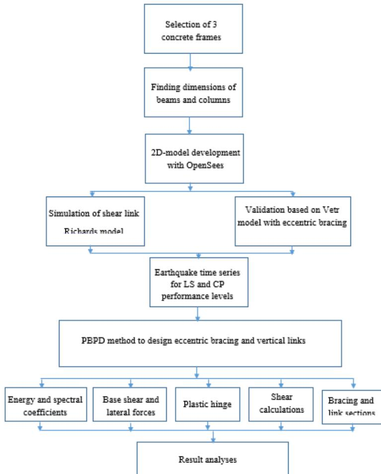
Fig. 7 Flow chart of the study considering PBPD for seismic rehabilitation
