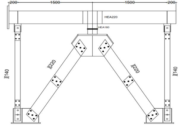
Fig. 4 Schematic layout of the frame with the bracing (Vetr 1998)
