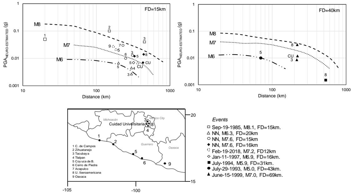
Fig. 8 Neural attenuation curves and a set of rock-like sites, validation cases
