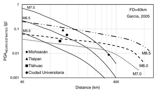
Fig. 15 Recordings during the September 19<sup>th</sup> 2017 event, comparison between the neural curves (dotted lines) and a GMPE (García *et al.* 2005) (continuous lines)
