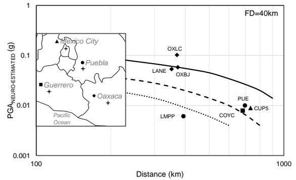
Fig. 14 Some registered PGAs during the September 8<sup>th</sup> 2017 event, the highest curve is for M8.5, the middle one is for M8 and the lowest is for M7.5
