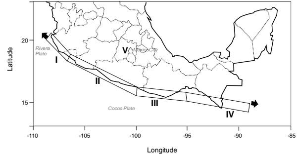
Fig. 3 Predefined seismic environments for Mexican subduction (modified from Ordaz and Reyes 1999)
