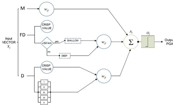
Fig. 5 NN structure: 3 inputs (two of them are a double-node), 1 hidden layer and 1 output
