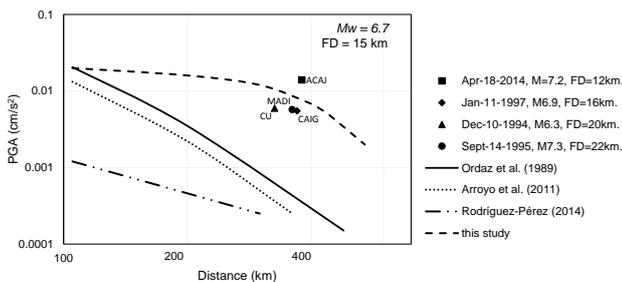
Fig. 9 Comparison of the attenuation curves from this study and some other for interplate earthquakes in central Mexico
