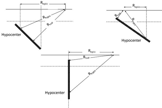
Fig. 2 Illustration of various measures of distance to fault rupture plane for dipping and vertical faults (modified from Gupta 2006)
