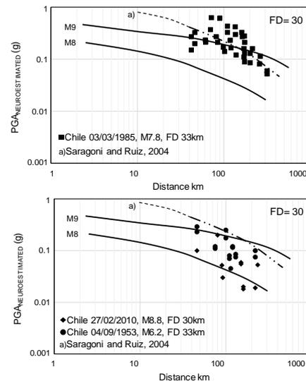
Fig. 11 Comparison between Chilean GMPE and the NN attenuation curves
