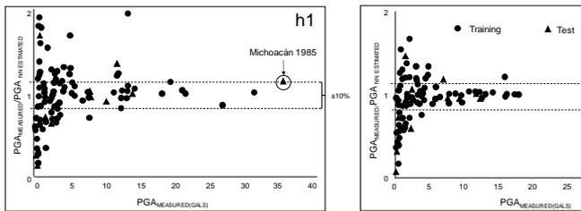
Fig. 6 Measured and Calculated PGA's, training and testing cases (triangle symbol points to the devastating earthquake of 1985, which is a test case)
