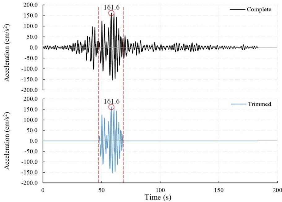
Fig. 2 Accelerometric record for the September 19, 1985 earthquake, for SCT site ( $T_g=1.9s$ ) in Mexico City lakebed. Complete record (upper location) and trimmed record (bottom)
