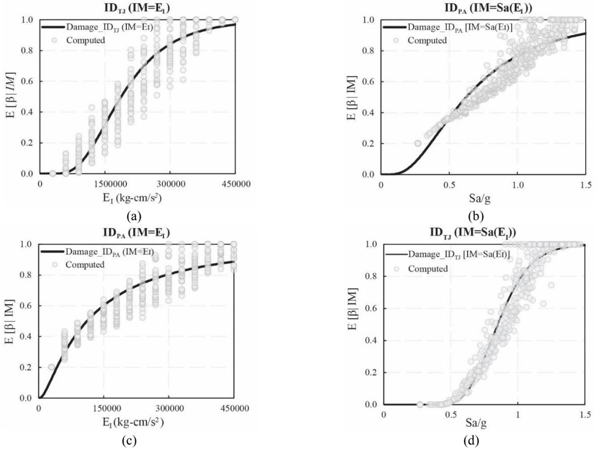
Fig. 6 Damage curves for SCT site ( $T_g=1.9s$ ). (a) and (c) for the Expected damage using  $E_I$  as objective IM, using (a) the damage models of Terán and Jirsa ( $ID_{TJ}$ ) and (b) Park and Ang ( $ID_{PA}$ ); expected damage using  $Sa$  as intensity measure, computed for the same damage models used in figures (a) and (c)
