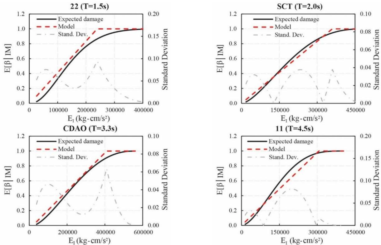
Fig. 14 Expected damage curves for different sites using both methodologies with their respective standard deviations
