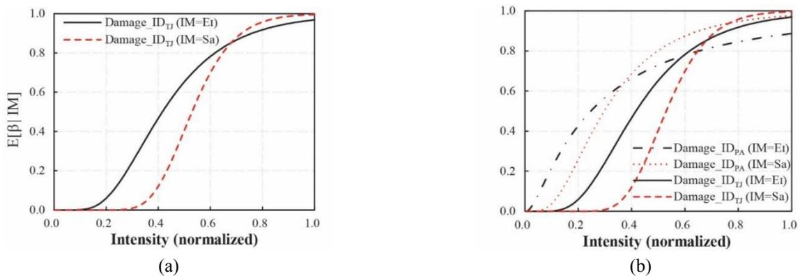
Fig. 8 Comparison of damage curves (normalized) considering different intensity measures ( $Sa$  and  $E_I$ )
