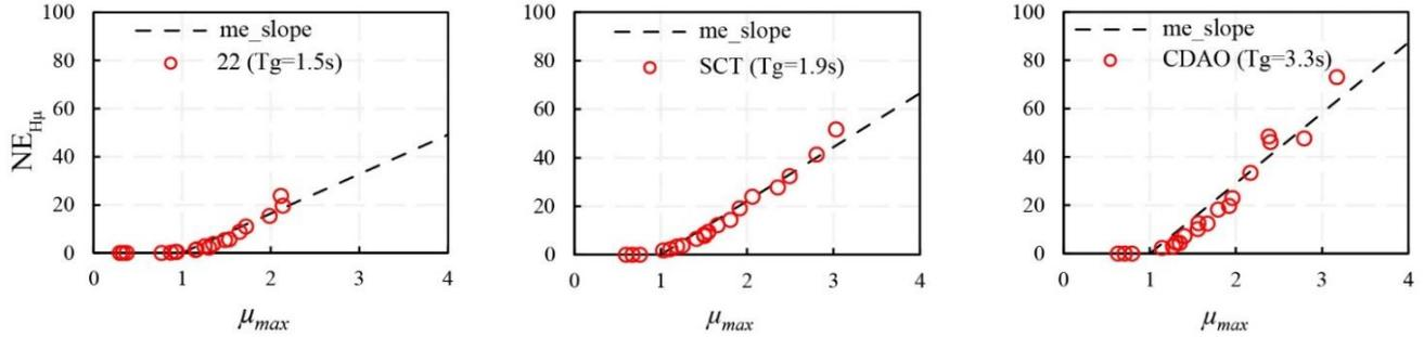
Fig. 9  $\mu_{\max}$ - $NE_{H\mu}$  relationship for an elasto-perfectly-plastic model for three different sites. The lateral strength was computed for  $Q=3.0$
