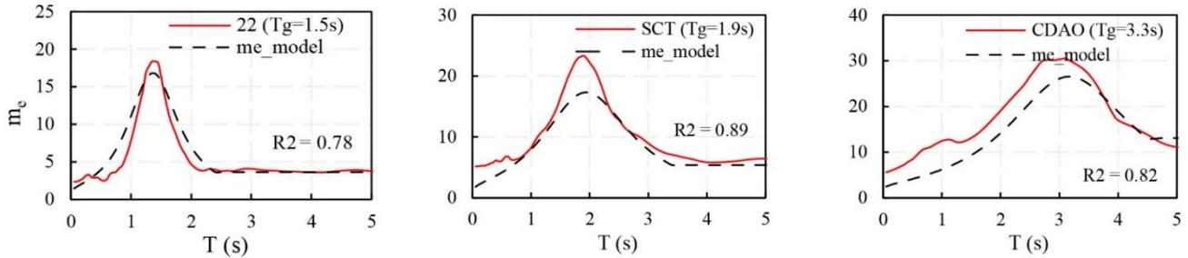
Fig. 10 Comparisons of the  $m_e$  model (dashed line) and the calculated values (continuous line) for three sites in the Mexico City, 22 ( $T_g=1.5s$ ), SCT ( $T_g=1.9s$ ) and CDAO ( $T_g=3.3s$ ), for a lateral strength computed with  $Q=3.0$
