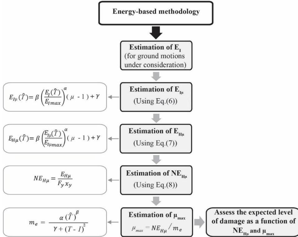
Fig. 11 Step-diagram for the energy-based methodology proposed in this article to evaluate accumulated and residual damage
