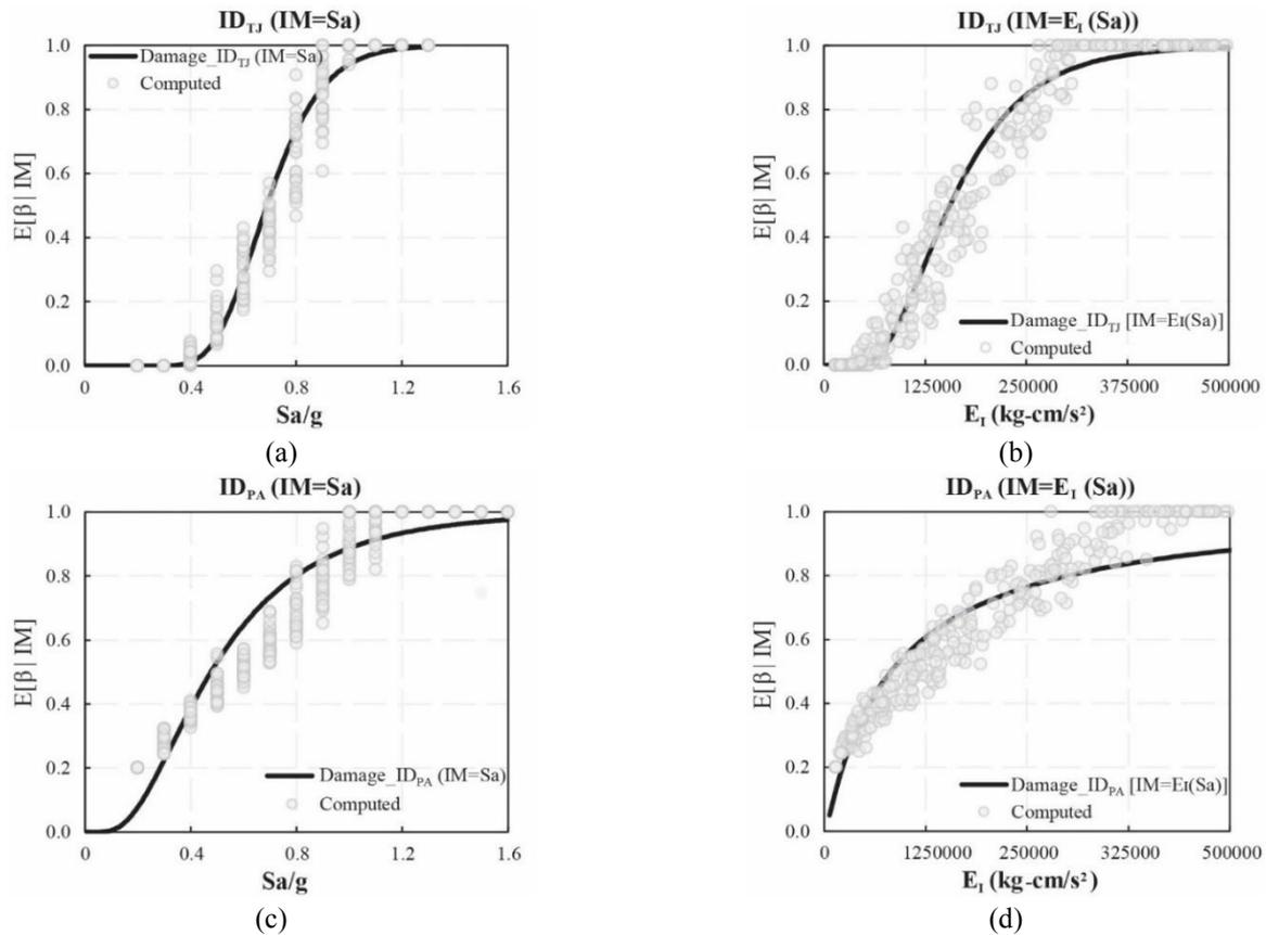
Fig. 7 Damage curves for SCT site ( $T_g=1.9s$ ). (a) and (c) for the expected damage using  $Sa$  as objective IM, using (a) the damage models of Terán and Jirsa ( $ID_{TJ}$ ) and (b) Park and Ang ( $ID_{PA}$ ); expected damage using  $E_I$  as intensity measure, computed for the same damage models used in figures (a) and (c)
