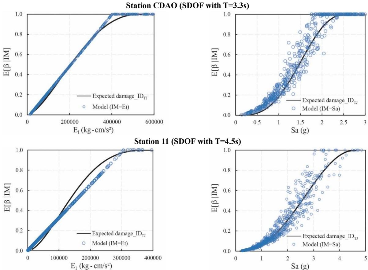
Fig. 13 Comparison of the expected damage computed with the energy-based proposed methodology (circles) and traditional non-linear methodologies (continuous line). For sites CDAO ( $T_g=3.3s$ ) and 11 ( $T_g=4.5s$ ) for SDOF systems stated in each figure and a  $Q=3.0$ . The Terán and Jirsa damage index was used
