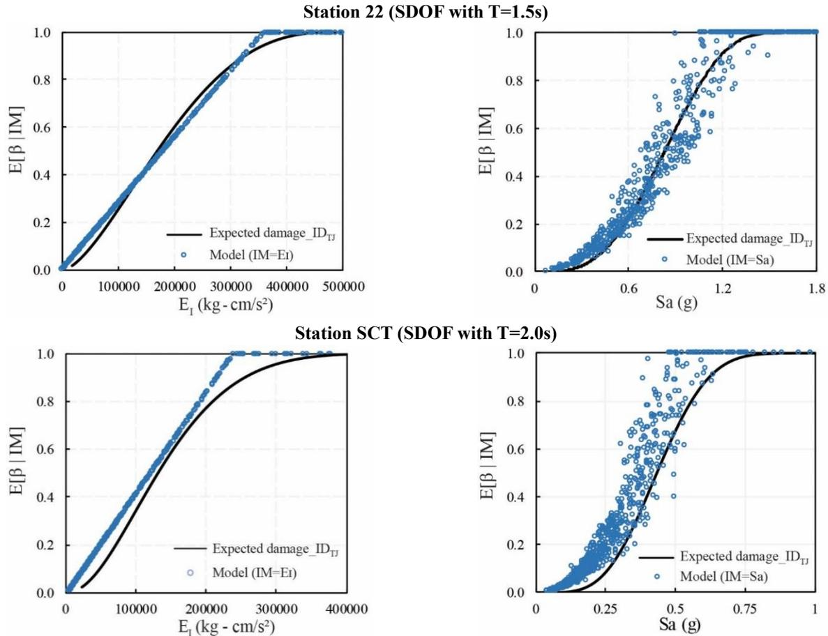
Fig. 12 Comparison of the expected damage computed with the energy-based proposed methodology (circles) and traditional non-linear methodologies (continuous line). For sites 22 ( $T_g=1.5s$ ) and SCT ( $T_g=1.9s$ ) for SDOF systems stated in each figure and a  $Q=3.0$ . The Terán and Jirsa damage index was used
