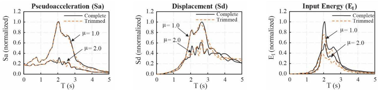
Fig. 3 Pseudoacceleration response spectra ( $S_a$ ), spectral displacement ( $S_d$ ) and input energy ( $E_I$ ). The spectra have been computed with the complete and trimmed records of Fig. 2, for elastic ( $\mu=1.0$ ) and nonlinear ( $\mu=2.0$ ) responses
