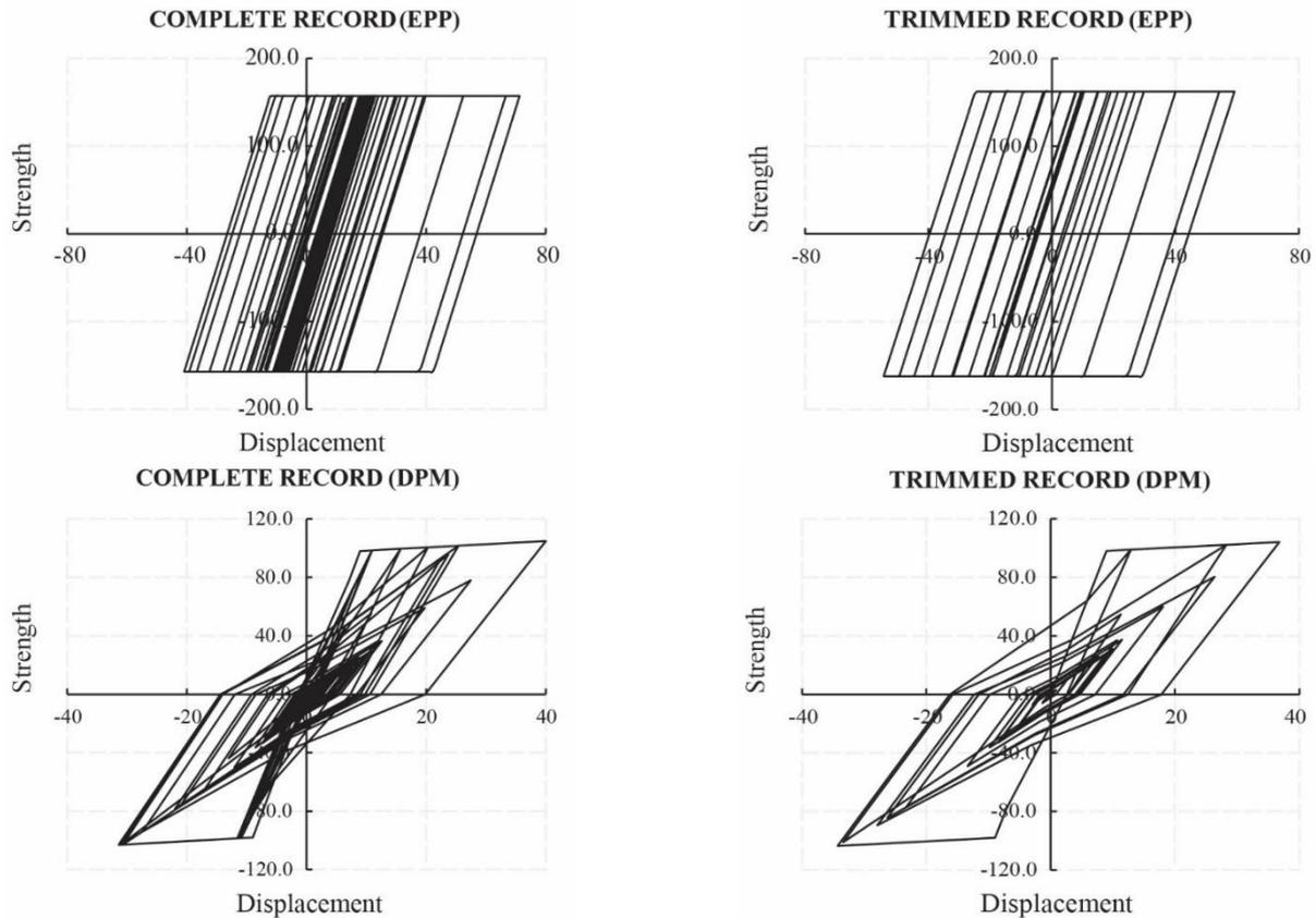
Fig. 4 Cyclic behavior for the complete and trimmed records of Fig. 2. The first row corresponds to elasto-perfectly-plastic behavior, the second one to stiffness degrading behavior
