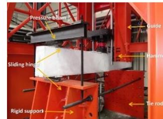
Fig. 4 Drop weight test set-up
