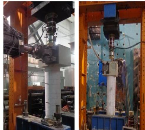
Fig. 10 Pier specimen and loading scheme
