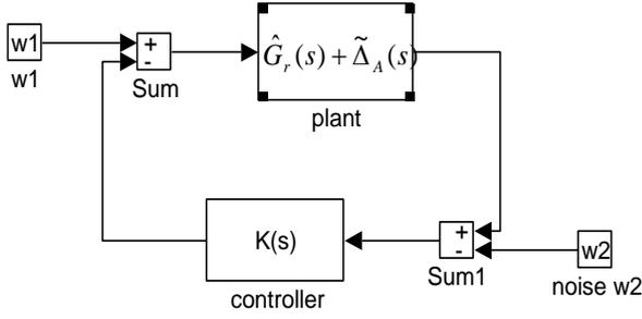
Fig. 2 Uncertainty representations for the active structural control system
