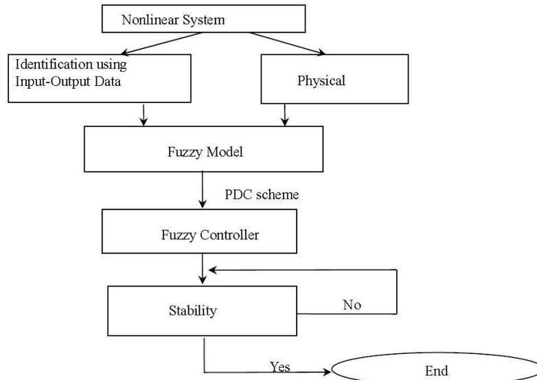
Fig. 1 Introduction the complete design procedure
