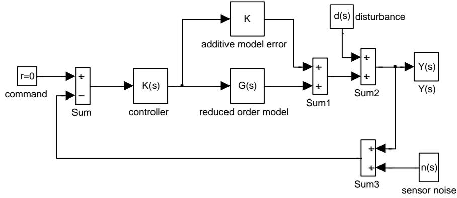
Fig. 3 The closed-loop configuration of the feedback control system
