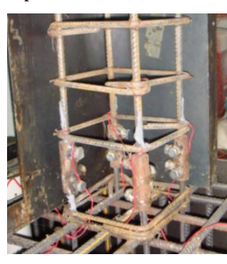
(d) Mechanical splices of reinforcement (screwlocks). Specimen M 1
