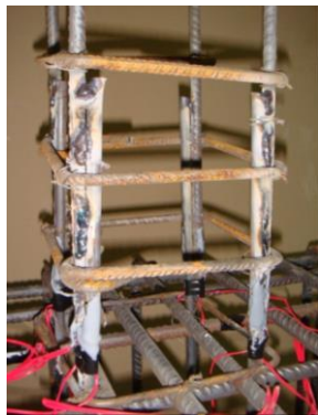
(a) Welded lap joint of reinforcing bars - type 1. Specimen W 1
