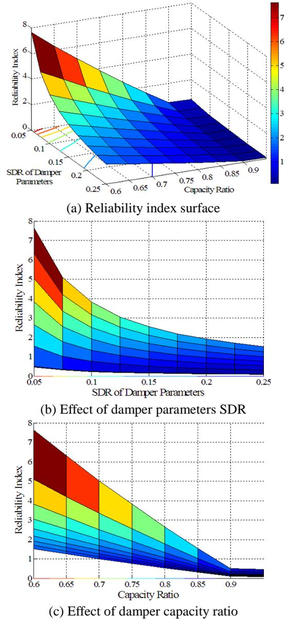
Fig. 8 Reliability Index ( $\beta$ ) variation against the variation of damper capacity ratio and standard deviation ratio for case study 2.
