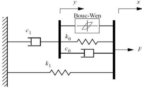
Fig. 2 Modified Bouc-Wen model of MR damper
