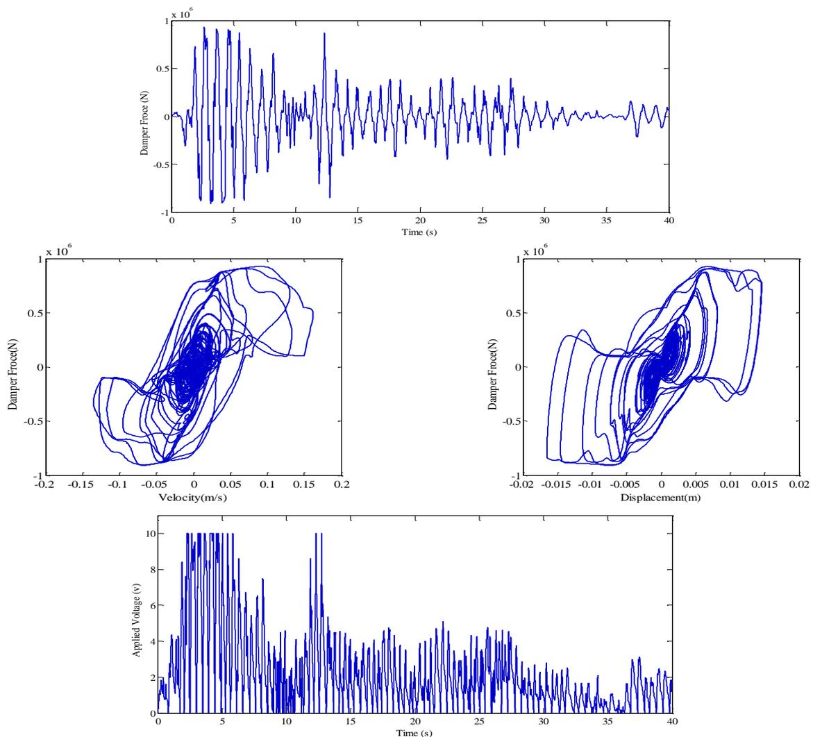
Fig. 3 Numerically obtained experimental data for the modified Bouc-Wen model, of a 1000 kN MR damper under the fuzzy control system simulation
