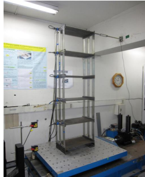
Fig. 8 Experimental configuration of a five-story shear frame (Koo et al. 2011)
