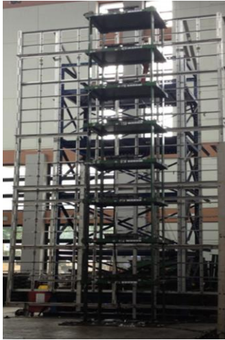
Fig. 12 Eight-story shear frame in the laboratory (Su et al. 2017)
