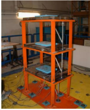
(a) Experimental configuration of shear frame
