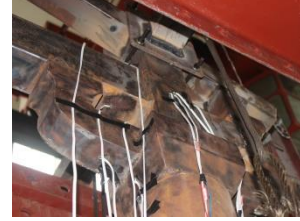
Fig. 10 Deformation of Dou-Gong of column Z-3 after test
