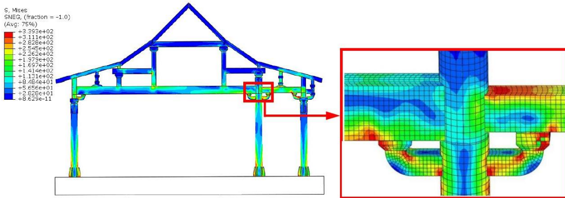
Fig. 23 Stress distribution under Wenchuan wave with the peak acceleration of 1000 gal
