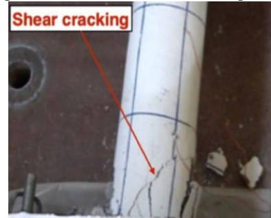
(b) The dilation of shear cracks results in gradual disintegration of the core concrete
