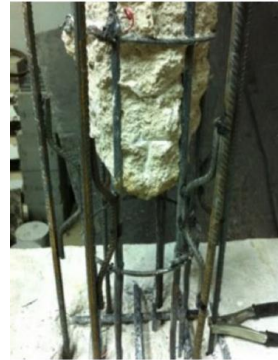
(c) S-shaped ( \sim ) segments were used to connect the longitudinal reinforcement of the RC jacket with the bars of the existing column
