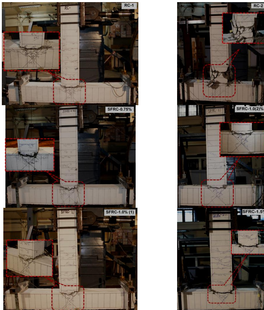
Fig. 7 Location of damages at the failure stage of specimens
