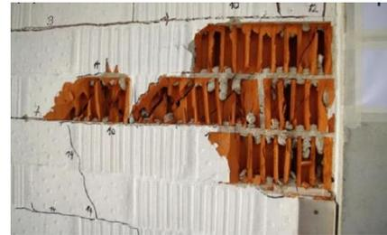
Fig. 5 Interlock effect in real structure (Penava 2012)
