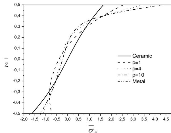
Fig. 3 The variation of the axial stress  $\bar{\sigma}_x$  through-the-thickness of a FG beam ( $L/h=2$ ) -Voigt model-
