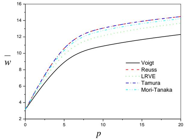
Fig. 2 The transverse displacement  $\bar{w}$  versus the power law index  $p$  of FG beams for different micromechanical models ( $L/h=5$ )
