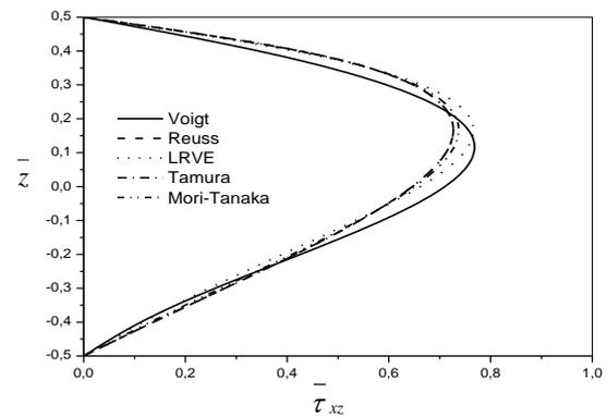
Fig. 6 The variation of the transverse shear stress  $\bar{\tau}_{xz}$  through-the-thickness of a FG beam for different micromechanical models ( $L/h=2, p=1$ )
