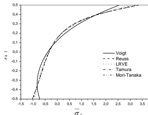
Fig. 4 The variation of the axial stress  $\bar{\sigma}_x$  through-the-thickness of a FG beam for different micromechanical models ( $L/h=2, p=1$ )
