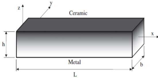
Fig. 1 Geometry and coordinate of a FG beam
