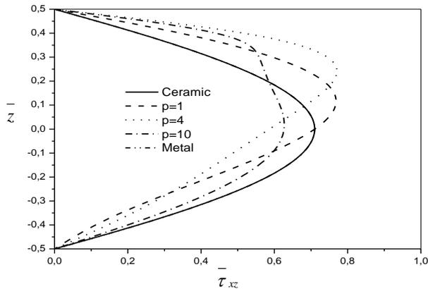
Fig. 5 The variation of the transverse shear stress  $\bar{\tau}_{xz}$  through-the-thickness of a FG beam ( $L/h=2$ ) -Voigt model-
