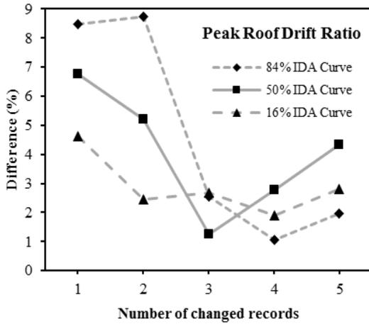
(a) The difference for IDA curves based on peak roof drift ratio
