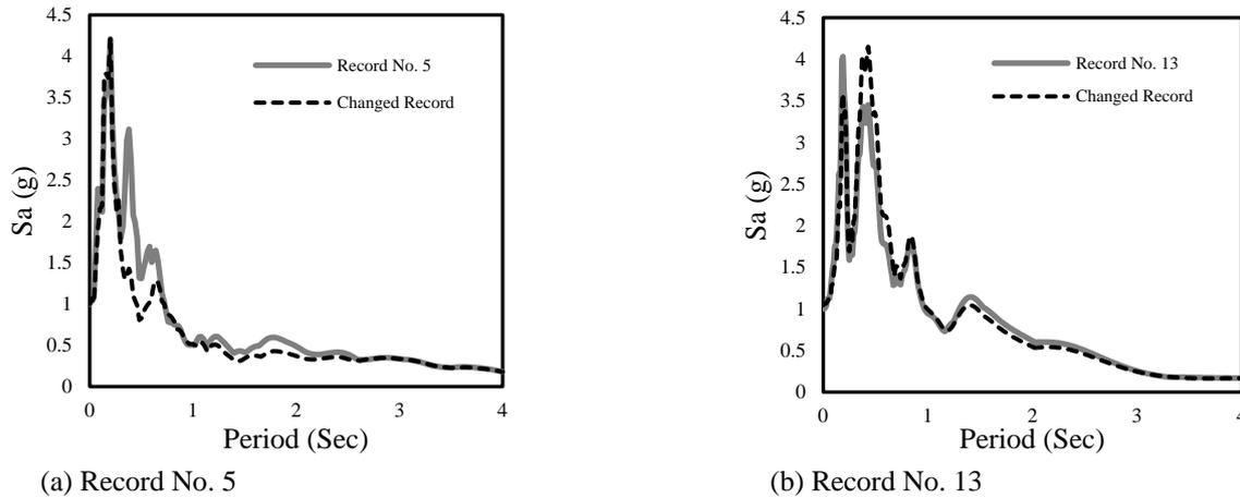
Fig. 8 Comparison between response spectra of first ground motion records with corresponding generated ground motion records
