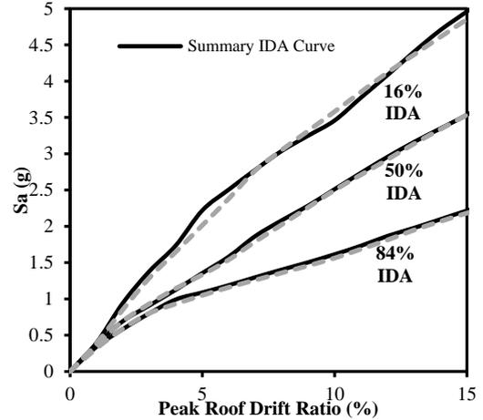
(a) IDA curves based on peak roof drift ratio
