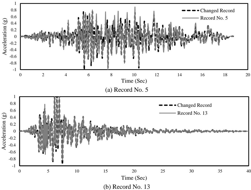
Fig. 9 Comparison between acceleration time histories of first ground motion records with corresponding generated ground motion records
