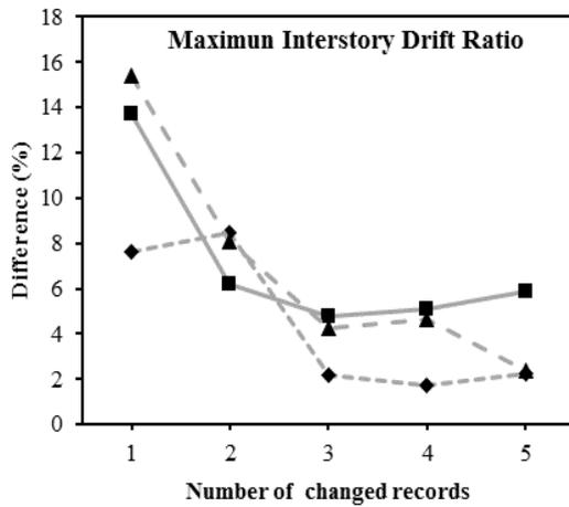
(b) The difference for IDA curves based on maximum inter-story drift ratio
