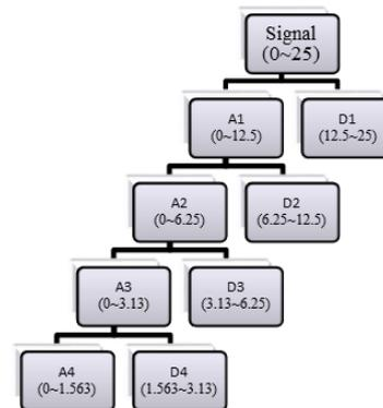
Fig. 1 Decomposing signal to 4 levels by DWT and their frequency range
