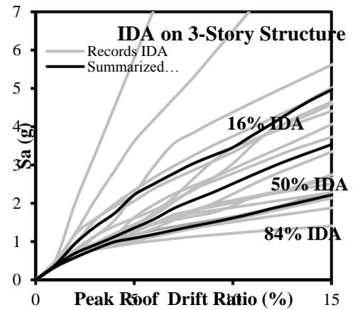
(b) IDA curves with 20 earthquake records and summarized fractiles
