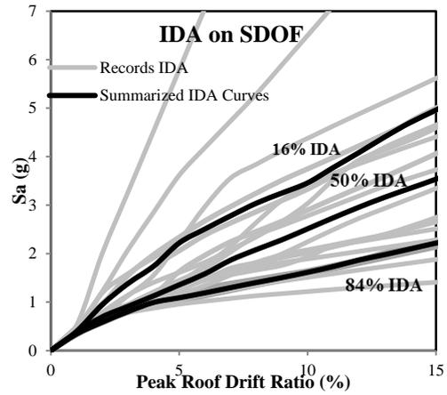
Fig. 6 IDA curves on SDOF system curves with 20 earthquake records and summarized fractiles
