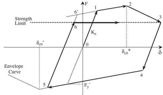
Fig. 5 Bilinear strength limit hysteretic behavior (Ibarra *et al.* 2005)
