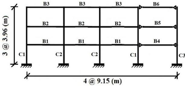
Fig. 2 Geometry of three-story special steel moment resisting frame
