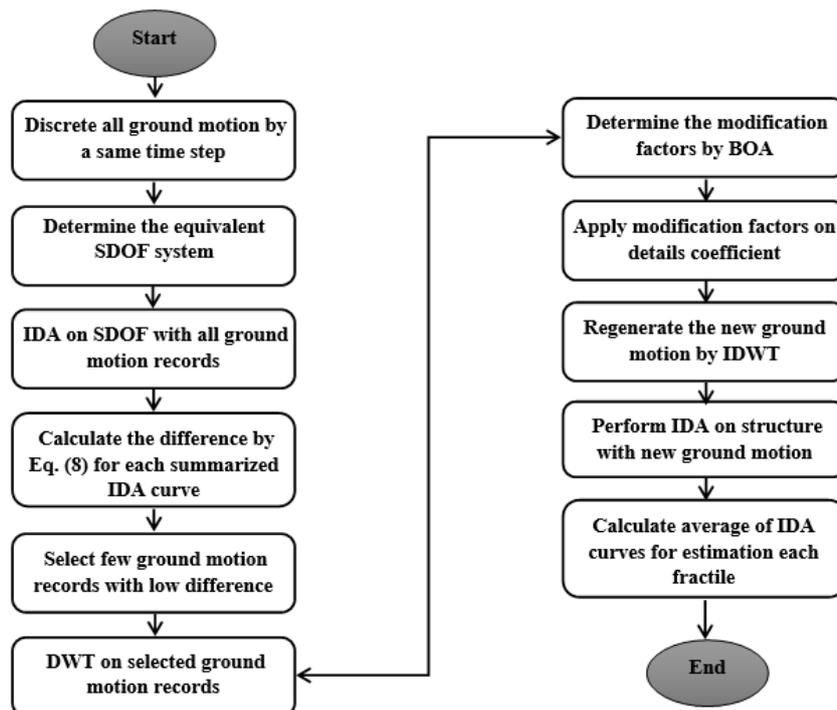
Fig. 7 Complete flowchart of suggested method
