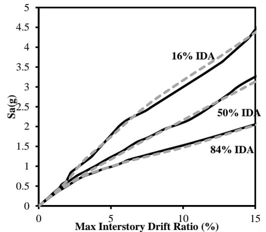
(b) IDA curves based on maximum inter-story drift ratio
