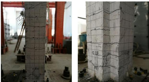
Fig. 7 Concrete cracks at column base
