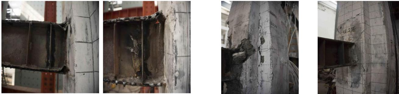
Fig. 6 Failure of beam-end
