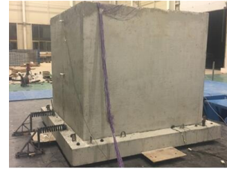
(b) Sliding isolation structure with spring-limiting devices
