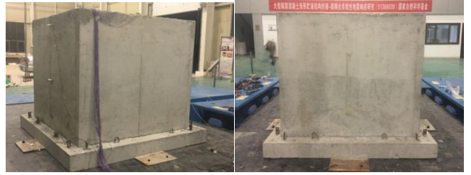
(c) Non-isolation concrete liquid-storage structure
