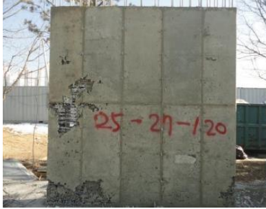
(b) Mock-up test of special shear wall (30-story residential building in Daegu, Korea)
