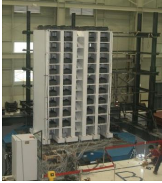
(b) Shake-Table test setup
