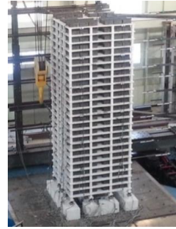
(a) Overview of the shaking table test setup
