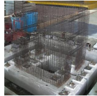
(d) Details of the core wall and the rebar fabrications of the core wall of the 1:15 scale model
