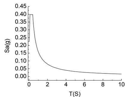
Fig. 3 The horizontal seismic design acceleration response spectrum under earthquake action E1
