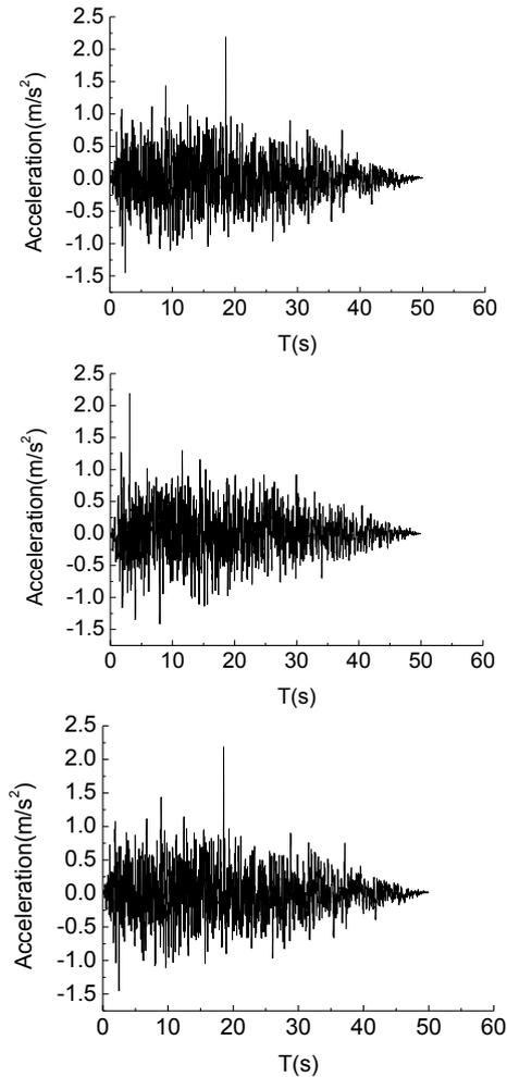
Fig. 4 Three artificial seismic acceleration time-history curves under earthquake action E1
