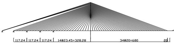
Fig. 6 The partially earth-anchored cable-stayed bridge scheme
