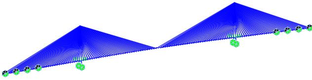
Fig. 2 3D dynamic finite element model of the example bridge
