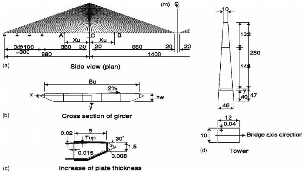
Fig. 1 General layout of a cable-stayed bridge with main span of 1400 m
