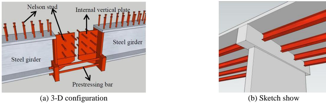
Fig. 1 Pier-to-deck connection joint (CCB)
