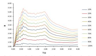
Fig. 2 Mean reduction of the elastic spectra due to damping.
