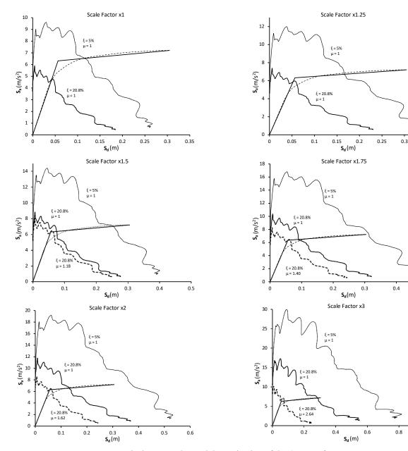
Fig. 8 Displacement demand determination of the 4-storey frame
