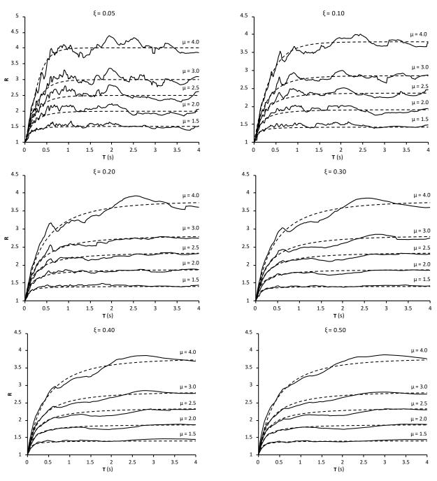
Fig. 4 Strength reduction factors R, by the analysis (solid line) and by the proposed relationships (dash line)
