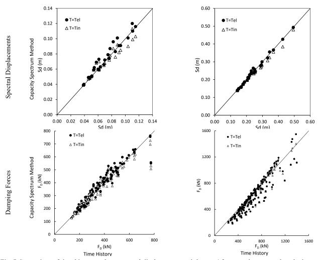
Fig. 7 Comparison of time history analyses spectral displacements and dampers' forces to the proposed method ones for the constant and adaptive damping assumptions (4-storey frame left and 6-storey frame right)
