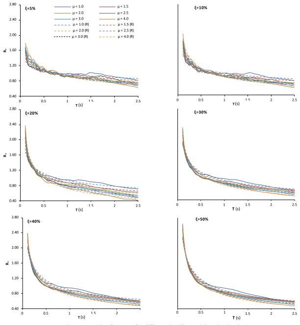
Fig. 5 Corrective factor B<sub>v</sub> for different ductility and damping levels
