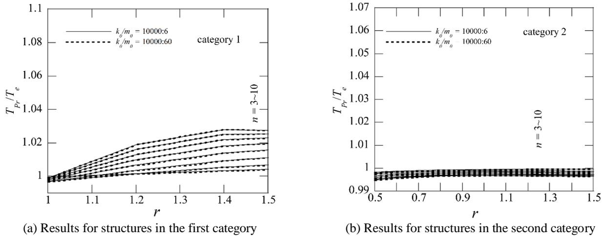
Fig. 5 Comparison between fundamental periods obtained by the proposed method and by eigenvalue analysis
