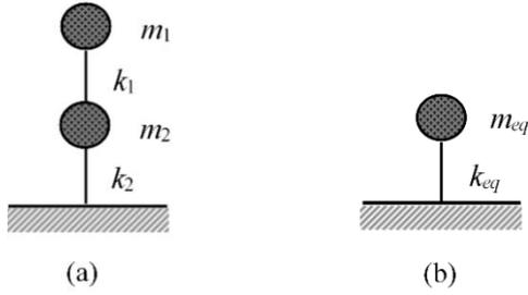
Fig. 1 Illustration of the concept of replacing a 2-DOF system with an equivalent SDOF system
