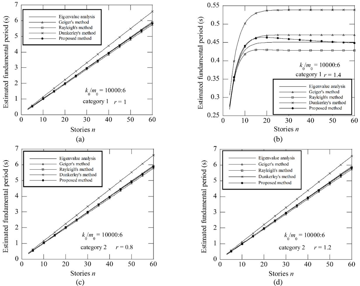
Fig. 6 Fundamental periods calculated by different methods. (a) Results for structures in the first category when  $r = 1$ . (b) Results for structures in the first category when  $r = 1.4$ . (c) Result for structures in the second category when  $r = 0.8$ . (d) Results for structures in the second category when  $r = 1.2$
