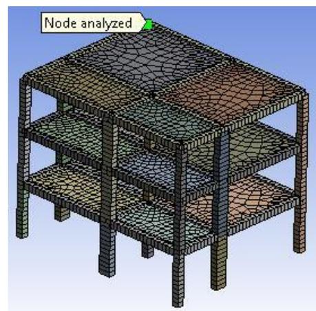
Fig. 4 Elevation view and Node selected to analyze of the dynamic behavior
