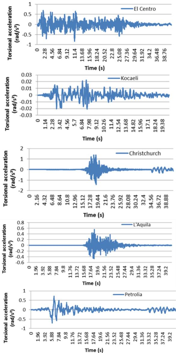
Fig. 1 Torsional time histories of the five earthquakes
