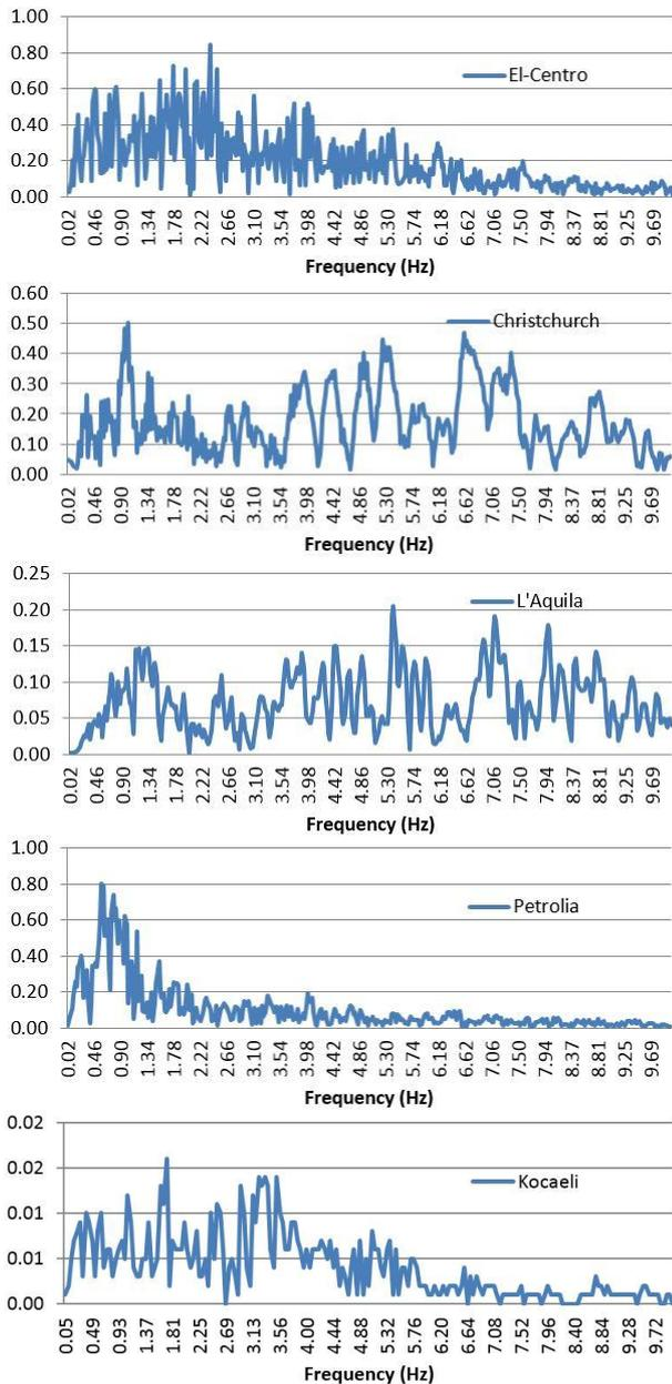
Fig. 2 Torsional acceleration Fourier spectrum
