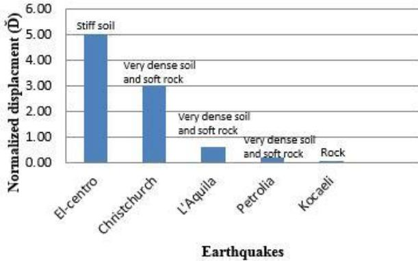
Fig. 6 Effect of different soil conditions on normalized displacement
