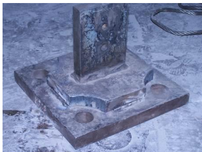
Fig. 3 Connection parts for boundary conditions B4 to B6
