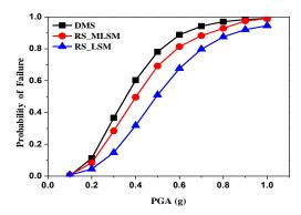
Fig. 4 Comparison of fragility curves for SDOF system (allowable displacements of 0.203 m)
