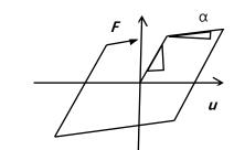
Fig. 1 (b) The force deformation behaviour of the nonlinear spring
