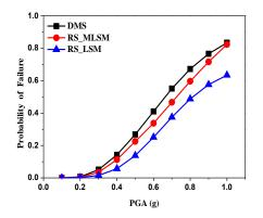
Fig. 5 Comparison of fragility curves for SDOF system (allowable displacements of 0.406 m)
