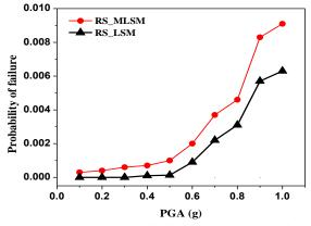
Fig. 11 Comparison of fragility curves of the considered building frame at CP level
