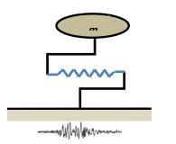
Fig. 1 (a) The spring mass system
