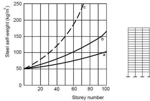
Fig. 2 Steel weight in multi-storey steel buildings (kg/m<sup>2</sup>) (a) Only due to vertical loads (b) Due to vertical and lateral loads (c) Only due to lateral loads
