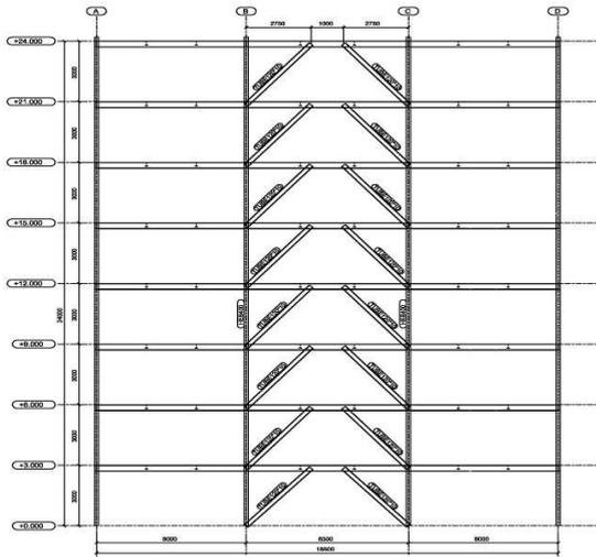
Fig. 4 Eccentric braced frames (Axis 1, 3 and 4) & (A, B, C and D)
