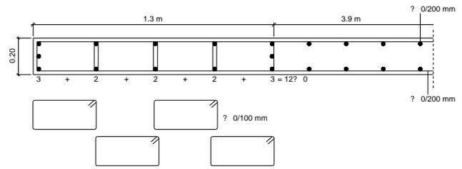
Fig. 9 Shear wall reinforcements
