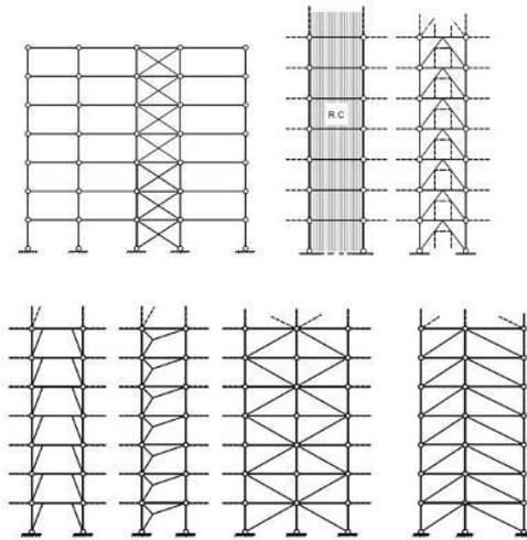
Fig. 1 Braced steel frames and reinforced concrete (RC) shear walls
