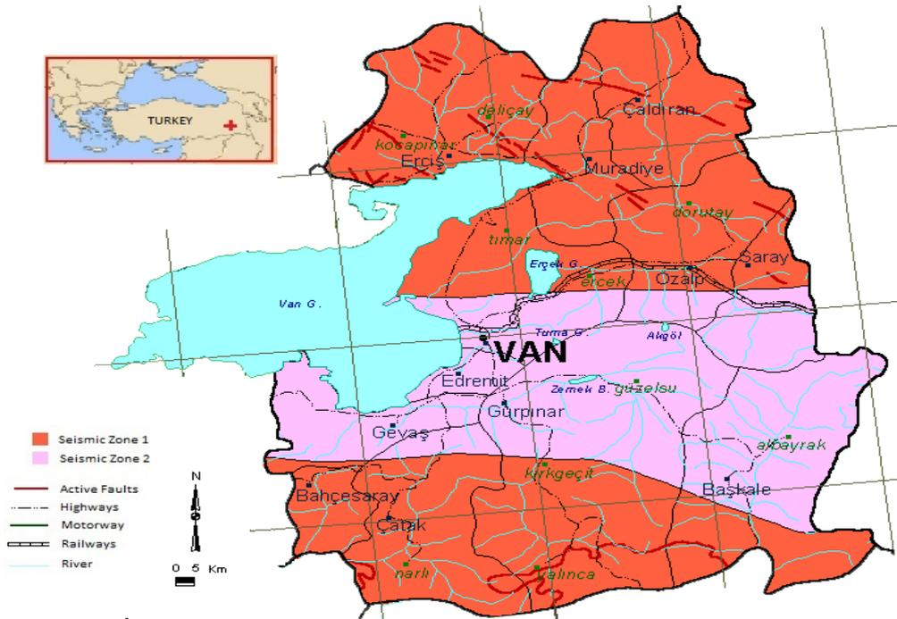
Fig. 2 Seismic Hazard Map of Van Region (where the red areas indicate the first degree zone with a minimum effective acceleration of 0.40 g and the pink areas mark the second degree zone with a minimum acceleration of 0.30 g
