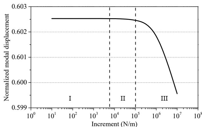
Fig. 10 Relationship between the normalized modal displacements of the beam-end and the changing in the support stiffness
