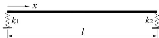
Fig. 5 Spring-supported Euler-beam model
