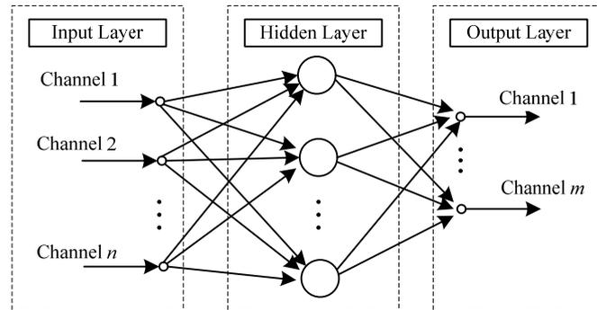
Fig. 1 Structure of the RBFNN
