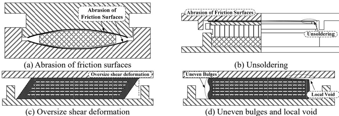
Fig. 4 Typical bearing damage
