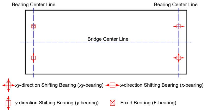
Fig. 12 Arrangement of the bearings
