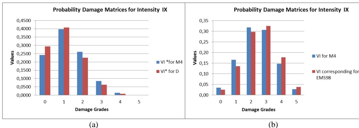
Fig. 12 Damage probability matrices for confined masonry for IX level of earthquake intensity: (a) using typological values ( $V_I^*$ ), (b) using Vulnerability index with added modifiers ( $V_I$ )
