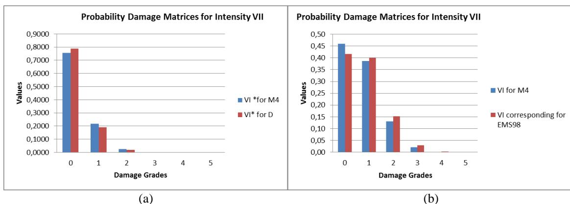
Fig. 10 Damage probability matrices for confined masonry for VII level of earthquake intensity: (a) using typological values ( $V_I^*$ ), (b) using Vulnerability index with added modifiers ( $V_I$ )
