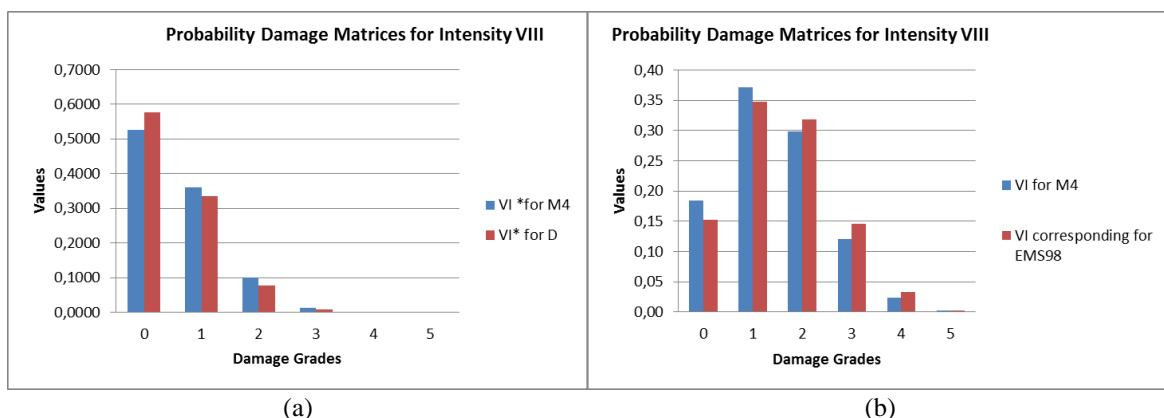
Fig. 11 Damage probability matrices for confined masonry for VIII level of earthquake intensity: (a) using typological values ( $V_I^*$ ), (b) using Vulnerability index with added modifiers ( $V_I$ )
