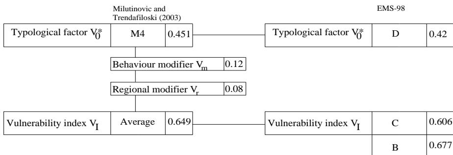
Fig. 8 Applied modifiers factors and corresponding vulnerability classes according to EMS-98
