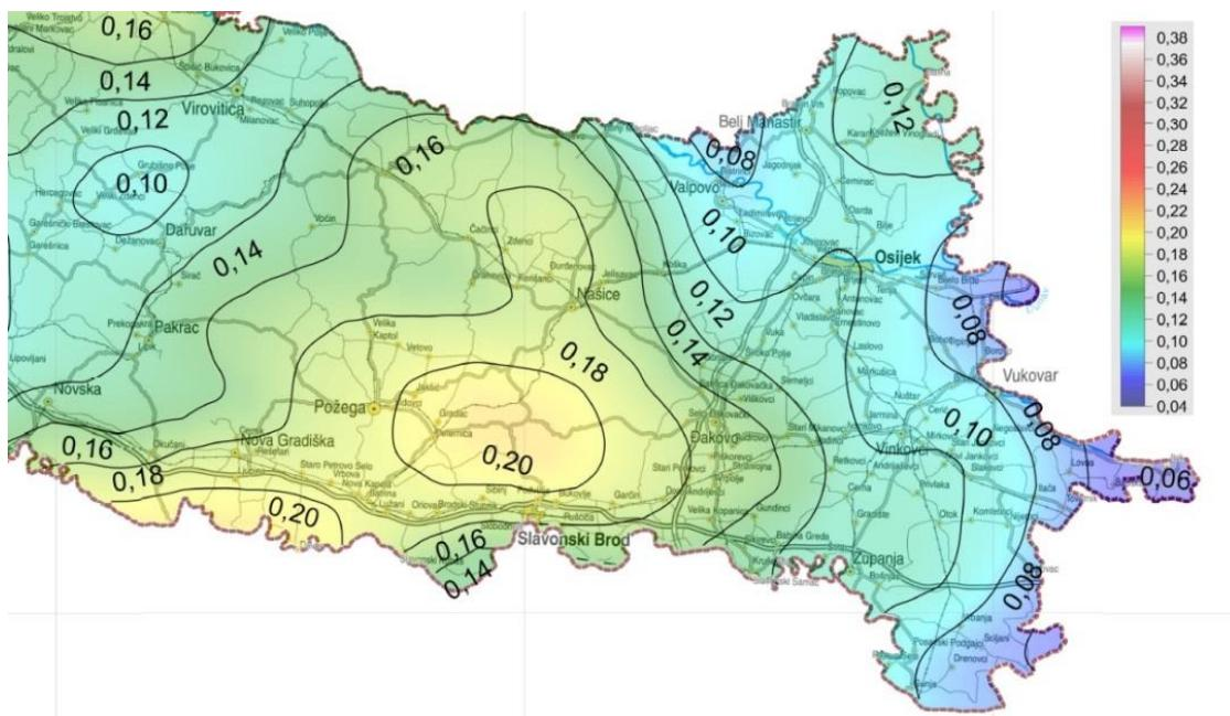
Fig. 4 Part of the Seismic hazard map for Croatia - map of Slavonia and Baranja (Herak 2012) for return period of 475 years
