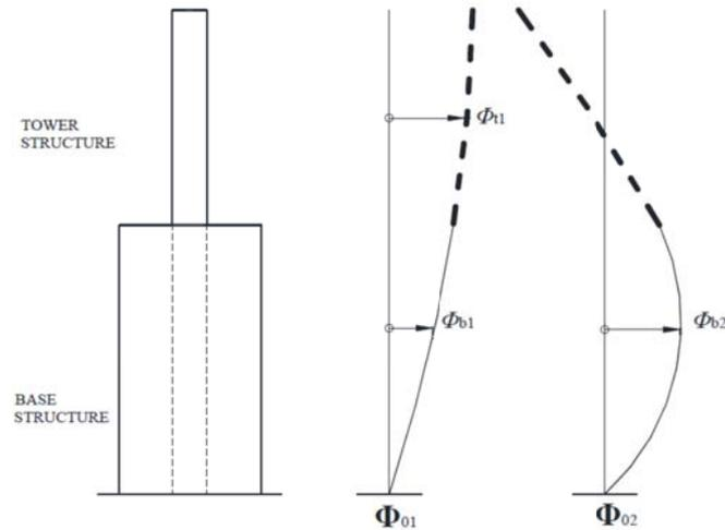
Fig. 2 The first two vibration shapes of a symmetrical setback building
