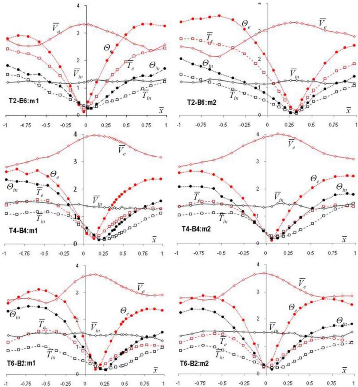
Fig. 6 Elastic and inelastic base shears, torques and top rotations ( $\times 10^{-2}$  rads) under the Kobe excitation
