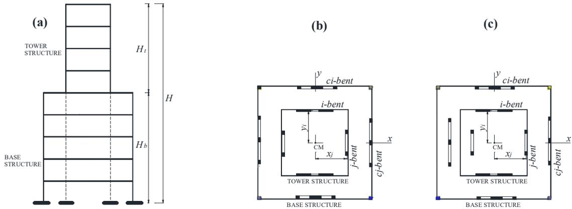
Fig. 1 (a) Multistory setback building with (b) a symmetrical plan configuration; (c) an asymmetric configuration
