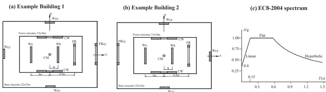
Fig. 3 (a),(b) Plan configurations of analyzed setback buildings; (c) Eurocode 8 acceleration spectrum
