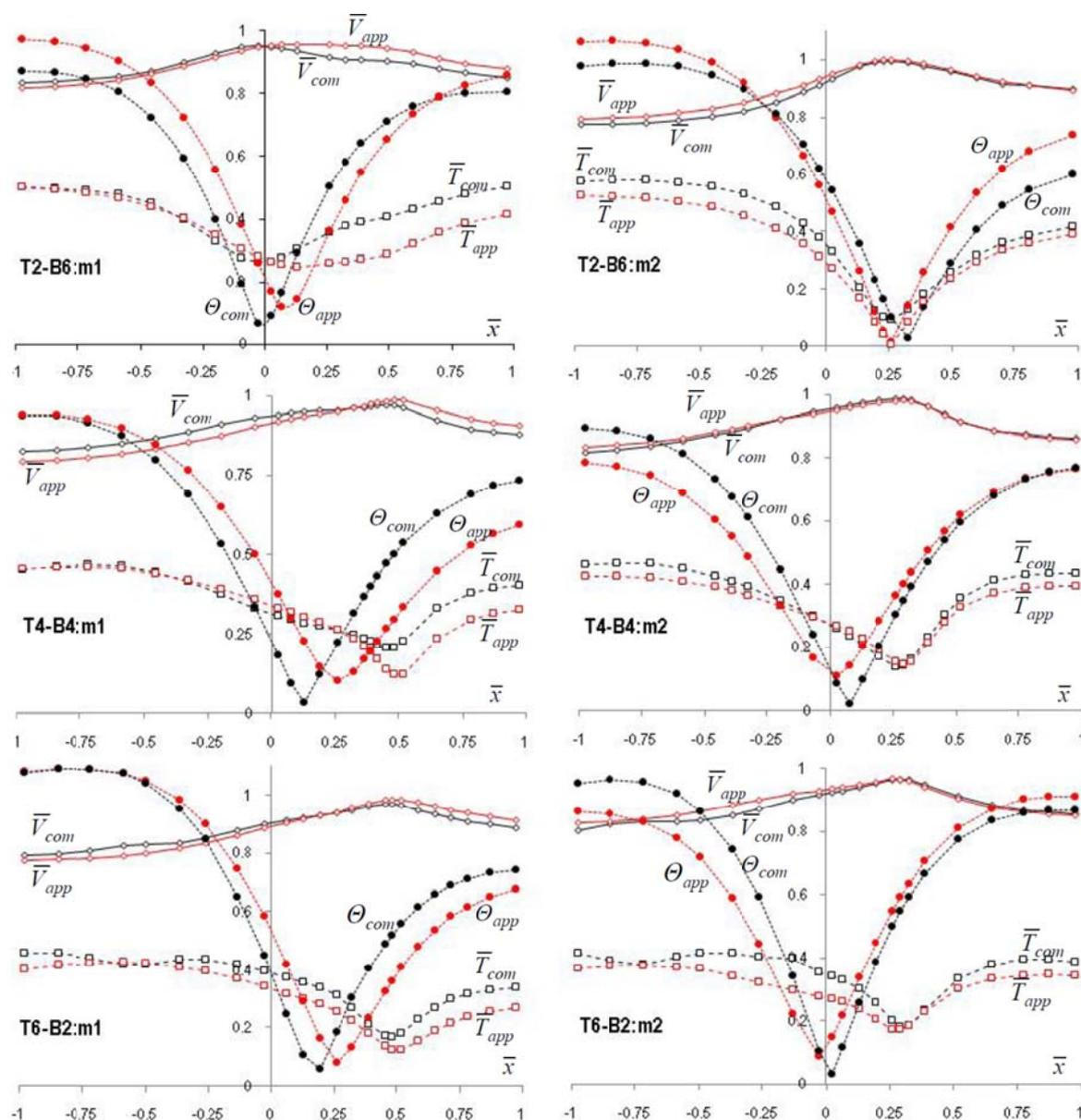
Fig. 5 Normalized elastic base shears, torques and rotations ( $\times 10^{-2}$  rads) of example buildings
