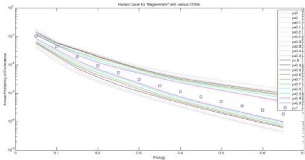
Fig. 13 The new method’s hazard curve for Baghershahr region with various DOMs
