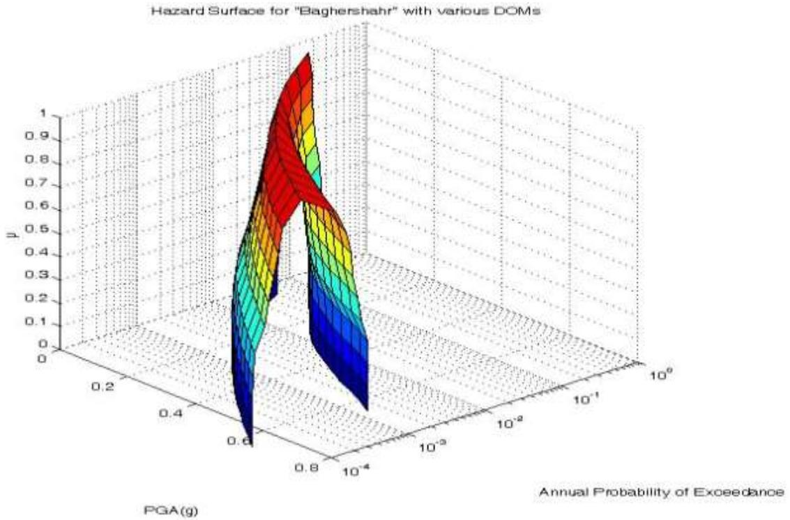
Fig. 14 The new method's hazard surface for Baghershahr region
