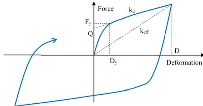
Fig. 2 Force - deformation relation of lead rubber bearings
