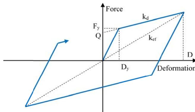
Fig. 1 Bilinear force - deformation relation of an isolator
