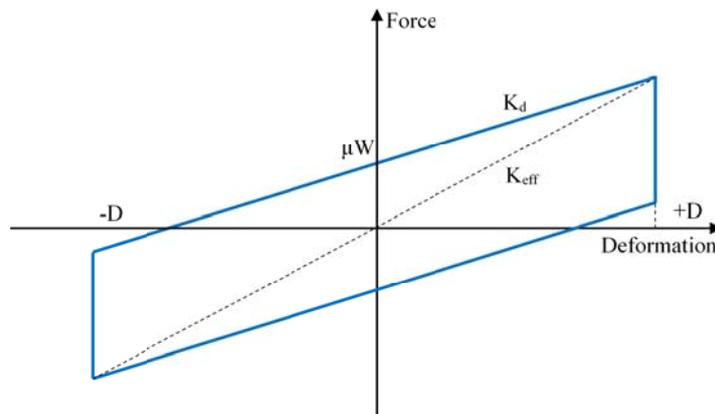
Fig. 3 Force - deformation relation of friction pendulum isolator
