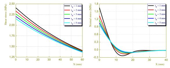
Fig. 19 Effect of adhesive layer thickness on interfacial stresses in reinforced concrete foundation beam repaired with Sika Carbodur composite plate
