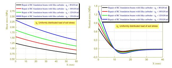
Fig. 10 Effect soil stress characteristics on interfacial stresses in reinforced concrete foundation beam repaired with Sika Carbodur composite plate
