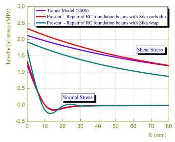
Fig 4 Comparison analytical results of interfacial stresses for composite plate repaired RC foundation beam
