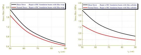
Fig. 8 Effect of height of the RC beam on interfacial stresses in reinforced concrete foundation beam repaired with composite plate
