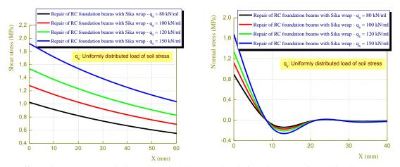
Fig. 9 Effect soil stress characteristics on interfacial stresses in reinforced concrete foundation beam repaired with Sika Wrap composite plate
