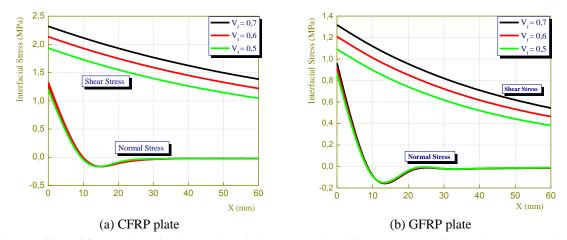
Fig. 14 Effect of fiber volume fraction on interfacial stresses in reinforced concrete foundation beam repaired with composite plate (a) CFRP plate and (b) GFRP plate
