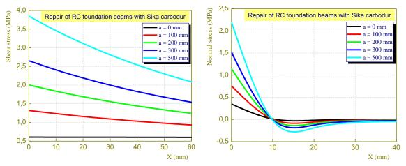
Fig. 13 Effect of the length of the repair plate  $L_p$  on interfacial stresses in reinforced concrete foundation beam repaired with Sika Carbodur composite plate
