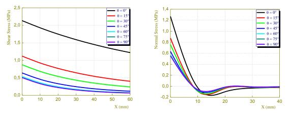
Fig. 15 Effect of fiber orientation on interfacial stresses in reinforced concrete foundation beam repaired with CFRP composite plate
