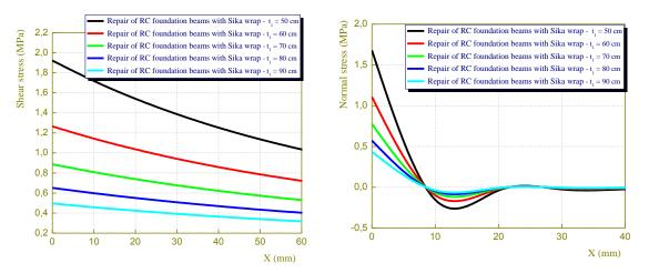
Fig. 6 Effect of rigidity of the RC beam on interfacial stresses in reinforced concrete foundation beam repaired with Sika Wrap composite plate
