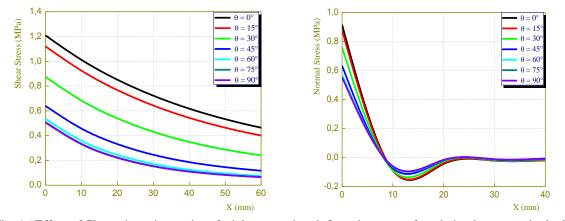
Fig. 16 Effect of fiber orientation on interfacial stresses in reinforced concrete foundation beam repaired with GFRP composite plate
