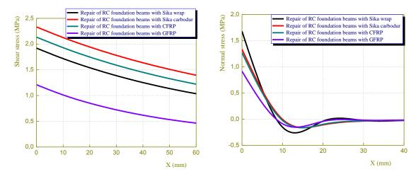
Fig. 5 Effect of plate stiffness on interfacial stresses in reinforced concrete foundation beam repaired with composite plate
