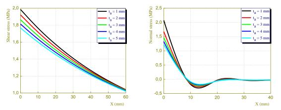
Fig. 18 Effect of adhesive layer thickness on interfacial stresses in reinforced concrete foundation beam repaired with Sika Wrap composite plate
