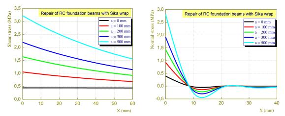
Fig. 12 Effect of the length of the repair plate  $L_p$  on interfacial stresses in reinforced concrete foundation beam repaired with Sika Wrap composite plate
