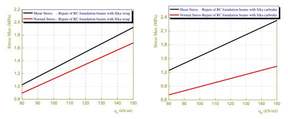
Fig. 11 Effect soil stress characteristics on interfacial stresses in reinforced concrete foundation beam repaired with composite plate
