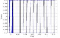
(a) stress-displacement perfect plasticity (friction damping)
