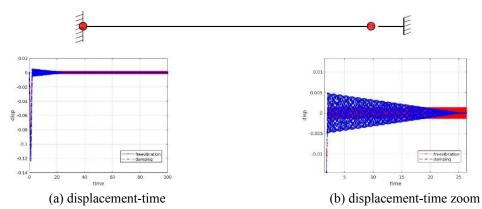
Fig. 9 Cantilever truss, oscillations displacement-time of free vibration and friction damping
