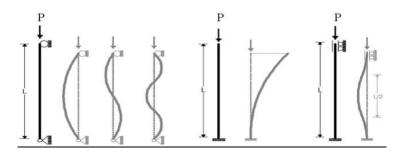
Fig. 4 Euler's buckling. (a) Simple supported (b) One fixed-one free end (c) Both end fixed beam
