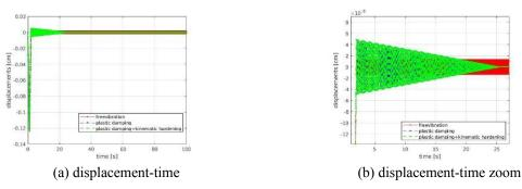
Fig. 10 Cantilever truss, oscillations displacement-time of free vibration, friction damping and kinematic hardening
