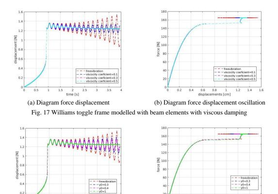
(a) Diagram force displacement (b) Diagram force displacement oscillation Fig. 18 Williams toggle frame modelled with beam elements with perfect plasticity damping
