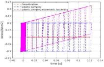
(b) stress-displacement perfect plasticity (friction damping) and kinematic hardening
