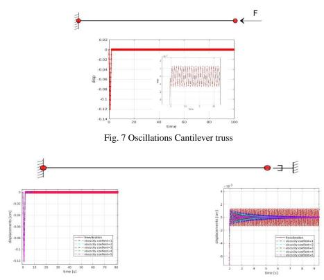
Fig. 8 (a) Cantilever truss with viscous damping, (b) oscillations changing viscosity coefficient
