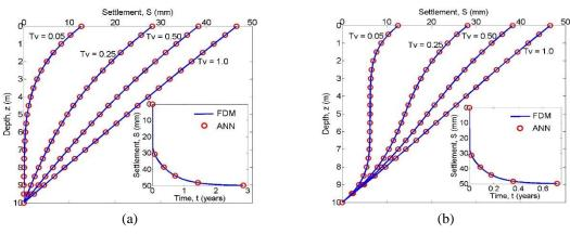
Fig. 12 Comparison of predicted settlements between FDM and ANN
