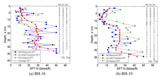
Fig. 7 Comparison of measured and predicted SPT-N and soil profiles
