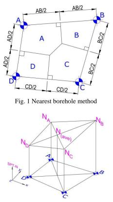
Fig. 2 Linear interpolation and spatial averaging method
