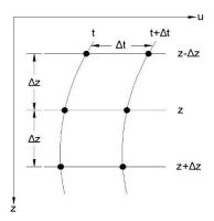
Fig. 8 Finite difference nodes in the numerical solution of the 1D consolidation equation
