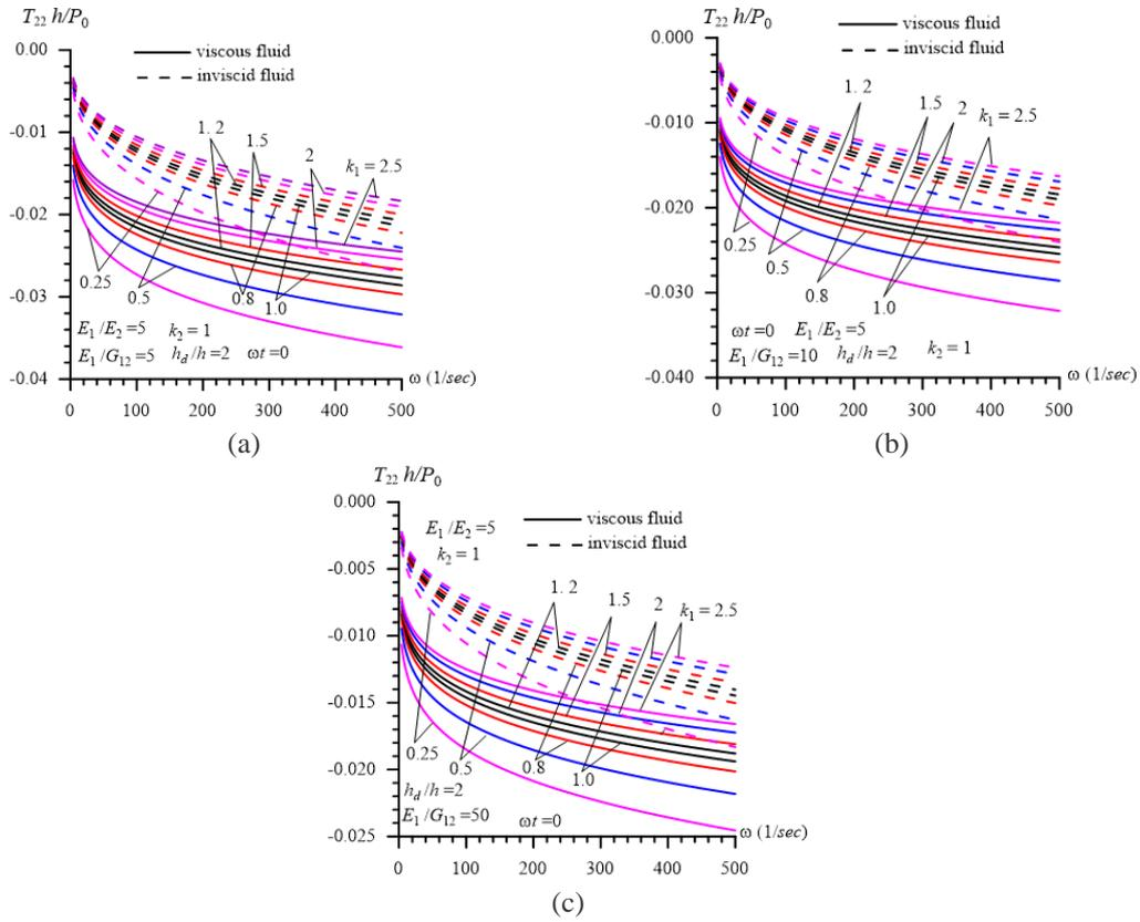
Fig. 5 The influence of the values  $k_1$  on the frequency response of the dimensionless interface stress  $T_{22}h/P_0$  in the cases where  $E_1/G_{12}=5$  (a), 10 (b) and 50 (c) under  $k_2=1$ ,  $\omega t=0$ ,  $h_d/h=2$  and  $E_1/E_2=5$
