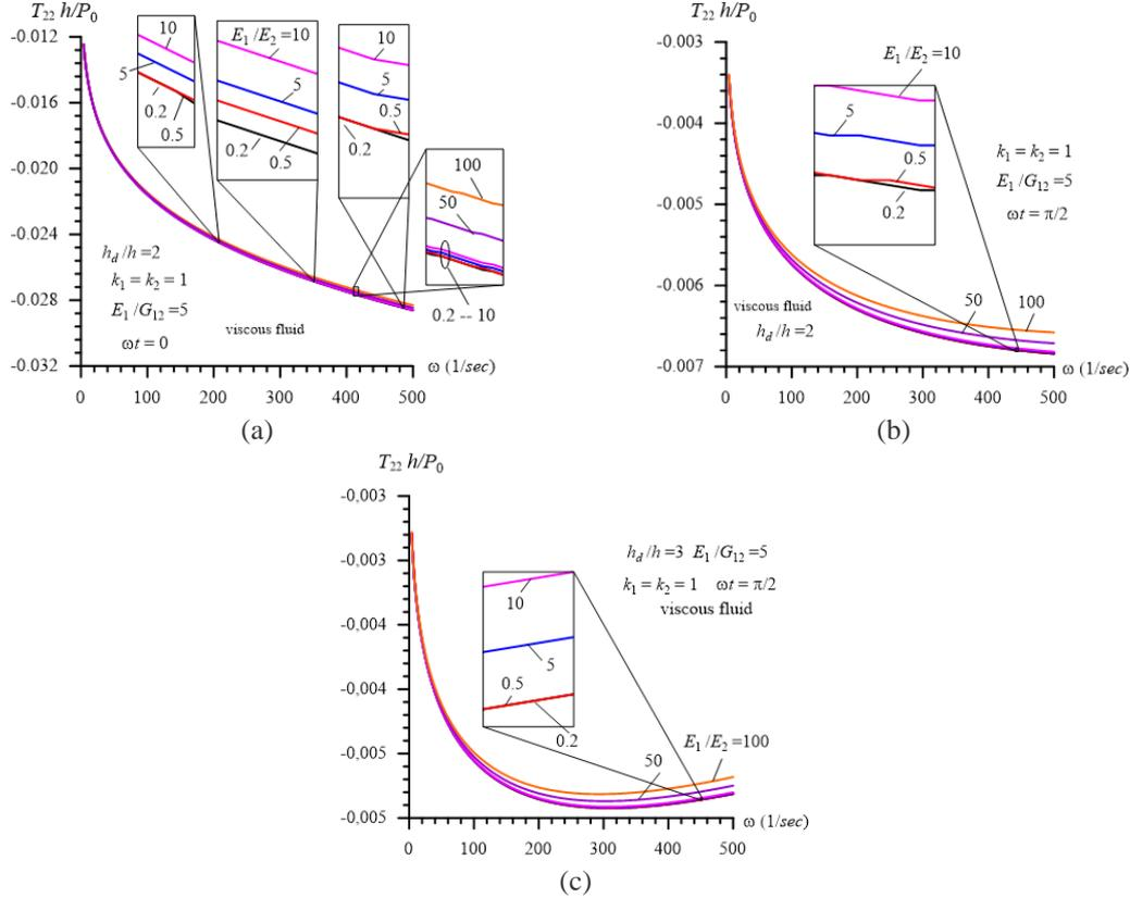
Fig. 4 Examples on the influence of the ratio  $E_1/E_2$  on the frequency response of the dimensionless interface stress in the case where  $k_1=k_2=1$ ,  $E_1/G_{12}=5$  under  $\omega t=0$ ,  $h_d/h=2$  (a);  $\omega t=\pi/2$ ,  $h_d/h=2$  (b) and  $\omega t=\pi/2$ ,  $h_d/h=3$  (c)
