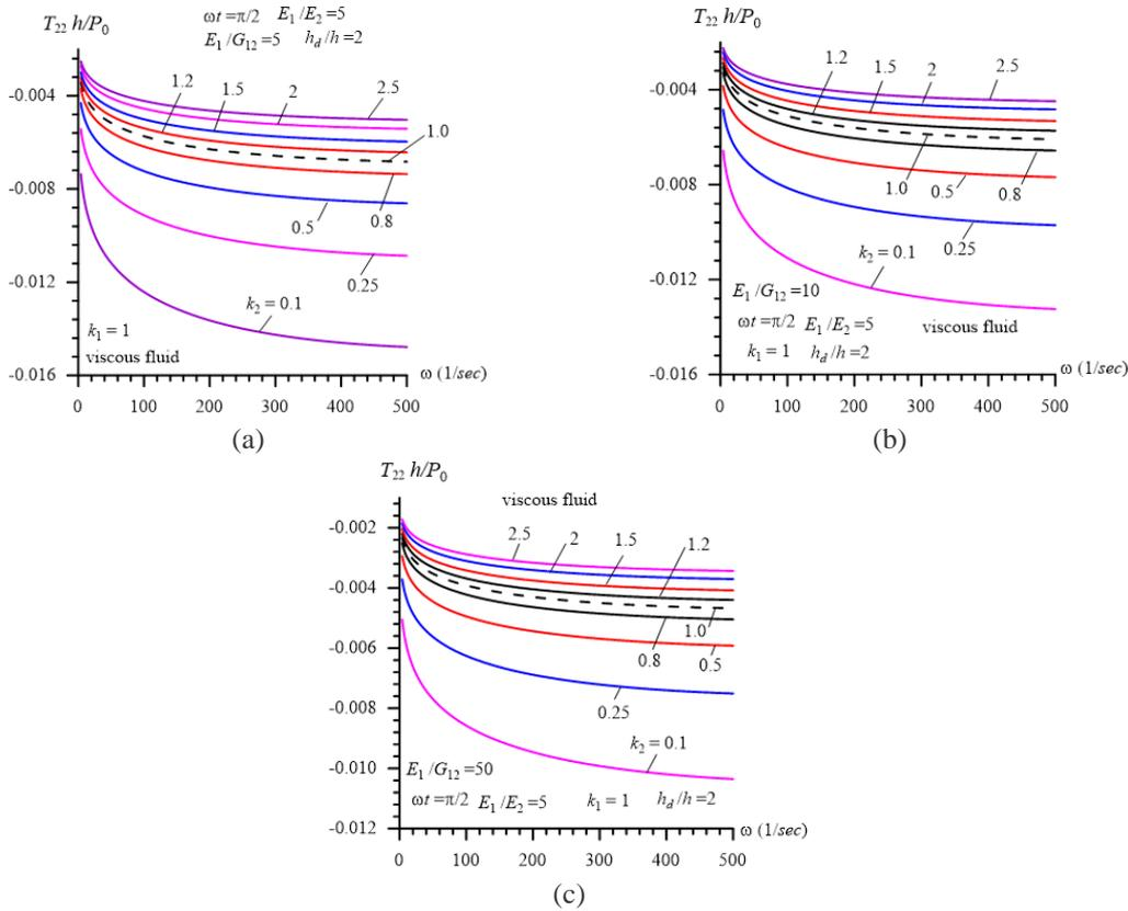
Fig. 8 The influence of the values  $k_2$  on the frequency response of the dimensionless interface stress  $T_{22}h/P_0$  in the cases where  $E_1/G_{12}=5$  (a), 10 (b) and 50 (c) under  $k_1=1$ ,  $\omega t=\pi/2$ ,  $h_d/h=2$  and  $E_1/E_2=5$
