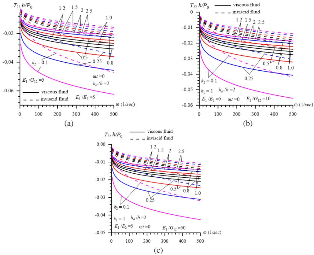
Fig. 7 The influence of the values  $k_2$  on the frequency response of the dimensionless interface stress  $T_{22}h/P_0$  in the cases where  $E_1/G_{12}=5$  (a), 10 (b) and 50 (c) under  $k_1=1$ ,  $\omega t=0$ ,  $h_d/h=2$  and  $E_1/E_2=5$
