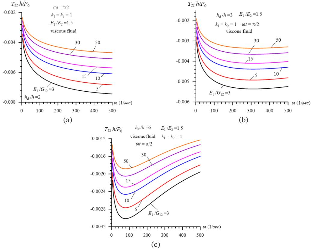
Fig. 3 The influence of the ratio  $E_1/G_{12}$  on the frequency response of the dimensionless interface stress  $T_{22}h/P_0$  in the case where  $\omega t = \pi/2$ ,  $k_1 = k_2 = 1$ ,  $E_1 = E_2 = 1.5$  under  $h_d/h = 2$  (a), 3 (b) and 6 (c)
