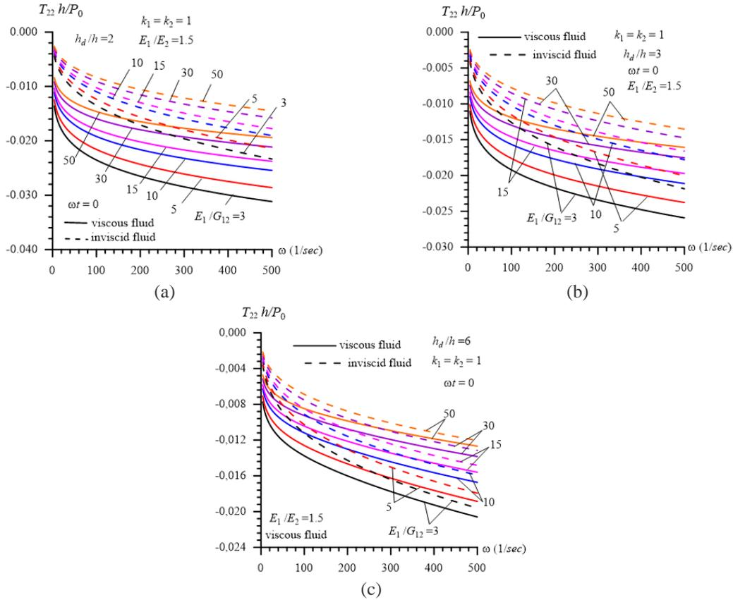
Fig. 2 The influence of the ratio  $E_1/G_{12}$  on the frequency response of the dimensionless interface stress  $T_{22}h/P_0$  in the case where  $\omega t=0$ ,  $k_1=k_2=1$ ,  $E_1/E_2=1.5$  under  $h_d/h=2$  (a), 3 (b) and 6 (c)
