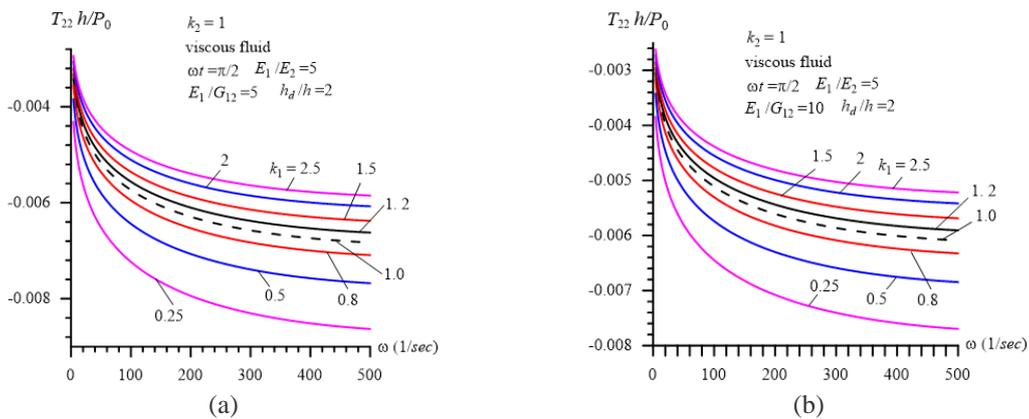
Fig. 6 The influence of the values  $k_1$  on the frequency response of the dimensionless interface stress  $T_{22}h/P_0$  in the cases where  $E_1/G_{12}=5$  (a), 10 (b) and 50 (c) under  $k_2=1$ ,  $\omega t=\pi/2$ ,  $h_d/h=2$  and  $E_1/E_2=5$
