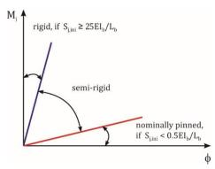
Fig. 2 Limits for stiffness classification of beam-to-column joints for unbraced frames (adapted from Eurocode 3-EN 1993-1-8 2005)
