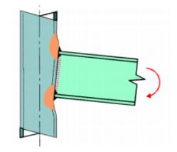
Fig. 3 Column wall plastification (adapted from CIDECT 2010)
