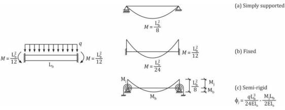
Fig. 1 Beam with various end conditions (adapted from CIDECT 2010)
