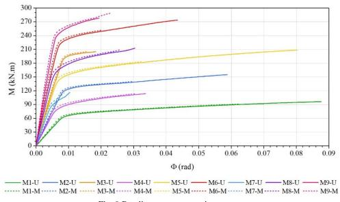
Fig. 9 Bending moment-rotation curves
