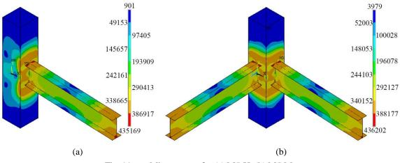
Fig. 11 von Miss stresses for (a) M5-U; (b) M5-M
