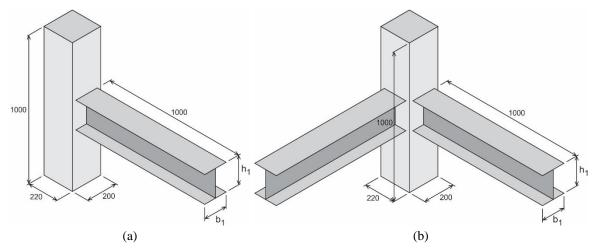
Fig. 4 Geometry and sizes of (a) uniplanar model; (b) multiplanar model. Units in mm
