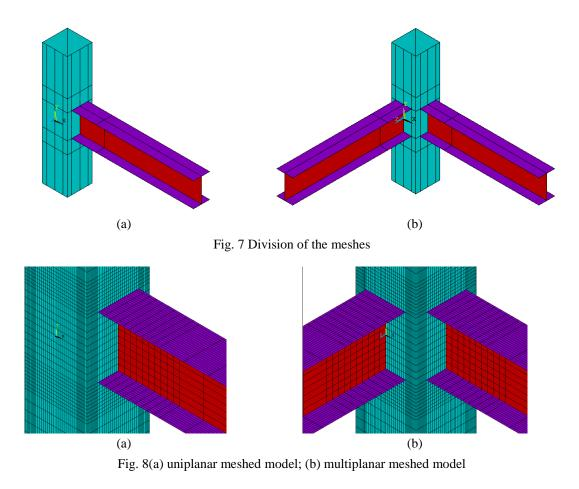
The application of boundary conditions consists in restricting all the six degrees of freedom in the nodes of the lower and upper extremities of the column, which will simulate fixed extremities. The following step was to apply a displacement of 50 mm in 100 increments at the end of the beams, with the aim of causing rotation in the welded connections and then plotting the moment-rotation curve.
