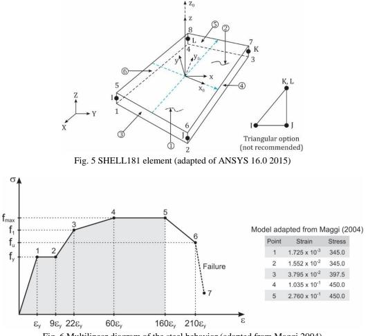
Fig. 6 Multilinear diagram of the steel behavior (adapted from Maggi 2004)
