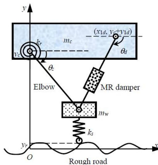
Fig. 1 Simplified model of torsion-bar suspension vehicle system
