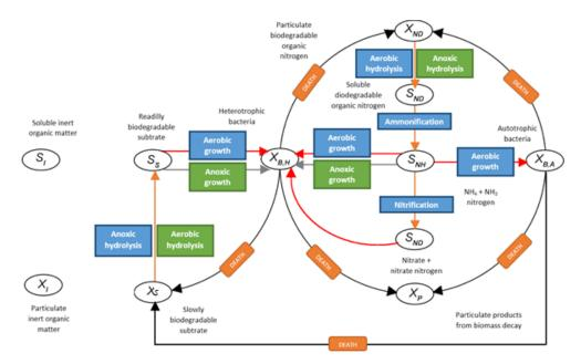
Fig. 3 Activated sludge model 1 - Model process
