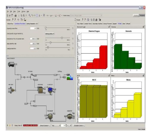
Fig. 5 GPS-X interface (GPS-X, 2008)
