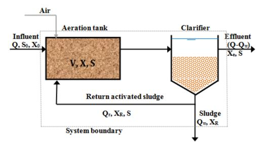
Fig. 1 Schematic diagram of activated sludge treatment process with model nomenclature with wasting from the sludge return line
