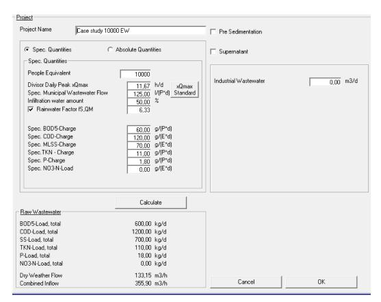
Fig. 7 AQUA DESIGNER - Calculation steps for WWTP (10.000 PE) (Aqua Designer, Software, 2010)
