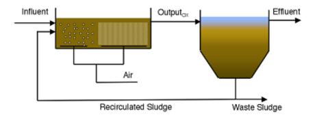
Fig. 2 Simple configuration for the activated sludge process
